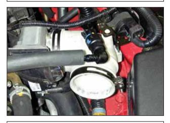
e. Slide the PSV onto the bracket previously installed on the EPDM coupler. Plug the plastic breather hose onto the nipple. Be sure both are secure before proceeding.
