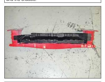
u. Remove the plastic splash shield from the bumper support.
