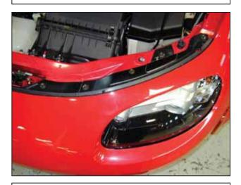
p. Remove the bolts securing the bumper to the radiator support on the driver side.
