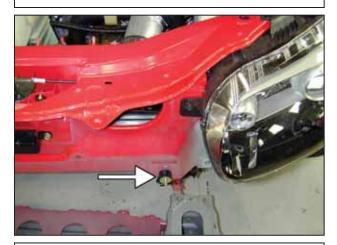
h. Install the supplied 5/8" rubber mount in the location shown. Secure using the supplied flat washer and nylock nut.
