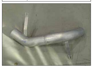
j. Ensure that the inside of the AEM® lower intake pipe is free and clear of any debris. Install the pipe into the reducing coupler on the upper intake pipe and align the pipe brackets with the rubber mounts. Once aligned, secure the pipe using a #9448 hose clamp.
