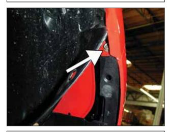
o. Remove the bolt securing the bumper to the passenger side fender where the fender liner was removed.
