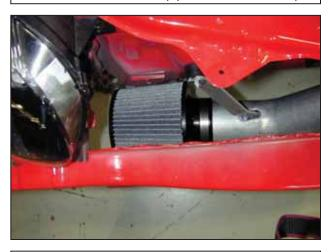
o. Position the AEM® intake for best fitment. Tighten the nuts on the mounting brackets. Re-adjust the pipe if necessary. Install the supplied filter sock to protect it from excess dust and water. NOTE: Please be aware the prefilter is water repellent, not water proof. Depending on conditions and usage the water repellent treatment is good for 1 to 2 years. See the parts list to reorder a new prefilter if necessary.
