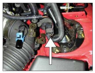
b. Slide the purge solenoid valve (PSV) toward the back of the car to remove it from the steel mount on the inlet hose. Unclip the wire harness.
