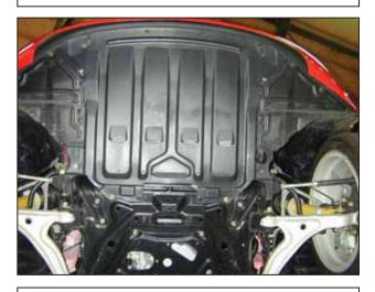
j. Remove the clips and bolts securing the center splash shield to the front bumper.
