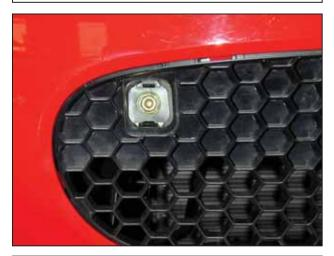
m. In the grill on the bumper there are two removable plastic covers. Remove these to reveal two bolts securing the bumper to the bumper support. Remove the two bolts.
