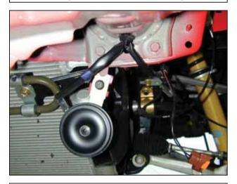
s. Unhook the wiring harness from the horn attached to the bumper support. Remove the 4 driver side bolts securing the bumper support to the chassis. Remove the plastic clips securing the plastic splash shield between the bumper support and the chassis.
