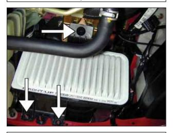
g. Remove the lower air filter housing and filter by removing the two nuts securing the housing to the chassis. Next, lift up on the back side of the housing and remove it from the vehicle.
