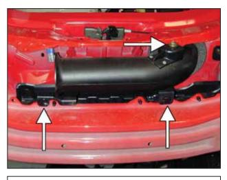
r. Remove the inlet air hose by removing the two retaining clips and the bolt securing it to the chassis.
