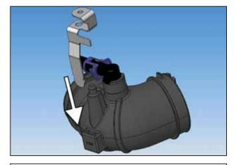
c. Install the steel PSV bracket from the stock inlet tube into the slot on the supplied EPDM coupler.
