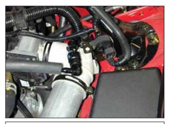
g. Ensure the inside of the AEM® intake pipe is free and clear of any debris. Install the upper intake pipe into the EPDM coupler on the throttle body. Secure using the stock hose clamp. Connect the MAF sensor connector to the MAF sensor.
