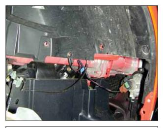
I. Remove the clips and bolts securing the passenger side front fender liner and remove the liner. Disconnect the fog light and side marker light from the wiring harness.
