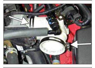
d. Remove the two stock hose clamps from the stock inlet tube and install them onto the EPDM coupler. Install the coupler onto the throttle body and secure.
