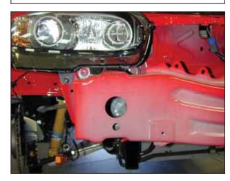
t. Remove the 4 remaining bolts securing the bumper support to the chassis on the passenger side. Remove the bumper support.
