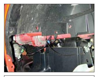
k. Remove the clips and bolts securing the driver side front fender liner and remove the liner. Disconnect the fog light and side marker light from the wiring harness.
