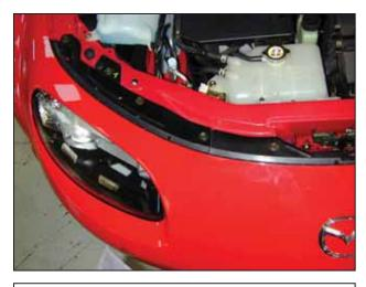
q. Remove the bolts securing the bumper to the chassis on the passenger side. Carefully remove the front bumper and set aside in a safe place.
