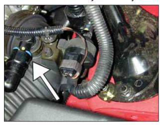
a. Unclip the hard plastic breather hose from the breather nipple by squeezing the blue retaining clip.
