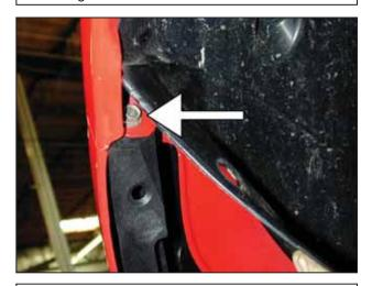
n. Remove the bolt securing the bumper to the driver side fender where the fender liner was removed.
