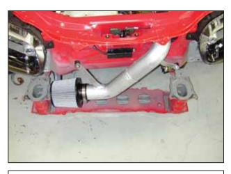
m. Install the AEM® air filter onto the end of the lower intake pipe. Push the air filter onto the inlet pipe until the stop in the filter is reached. Secure the air filter onto the inlet pipe with a hose clamp.
