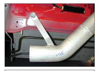
I. Secure the other pipe bracket using the remaining flat washer and nylock nut.
