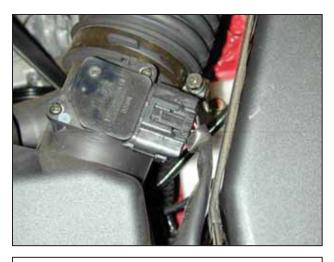
w. Remove the stock MAF sensor from the air filter housing. Be careful not to damage the MAF sensor.
