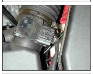
c. Unplug the MAF sensor from the wiring harness.
