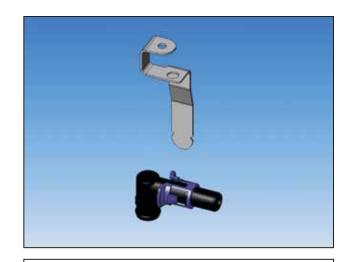
x. Remove the plastic breather nipple and the steel PSV bracket from the previously removed inlet tube.
