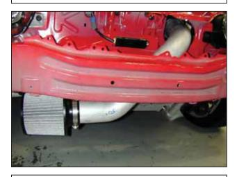
n. Install the front bumper support using the 8 previously removed bolts. Ensure the air filter does not contact any part of the vehicle.
