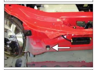
i. Install the other 5/8" rubber mount in the location shown. Secure using the supplied flat washer and nylock nut.
