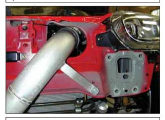
k. Secure the intake pipe bracket to the rubber mount using a flat washer and a 6mm nut.
