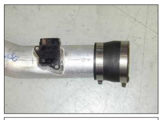
f. Install the MAF sensor into the upper intake pipe (2-704) and secure using the two supplied 8-32 bolts. Install the reducing coupler onto the end of the intake pipe and secure using the supplied #9444 hose clamp as shown.
