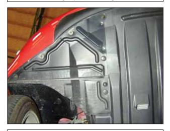
h. Remove the retaining clips and bolts securing the driver side splash shield to the bumper and chassis. Remove the splash shield.
