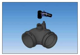
b. Install the plastic breather hose nipple from the stock inlet tube into the supplied EPDM coupler and secure using the stock spring clamp.
