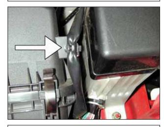
d. Unclip the MAF sensor wiring harness from the side of the air filter housing.
