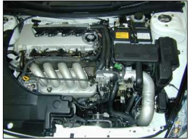
AEM® intake system installed.
