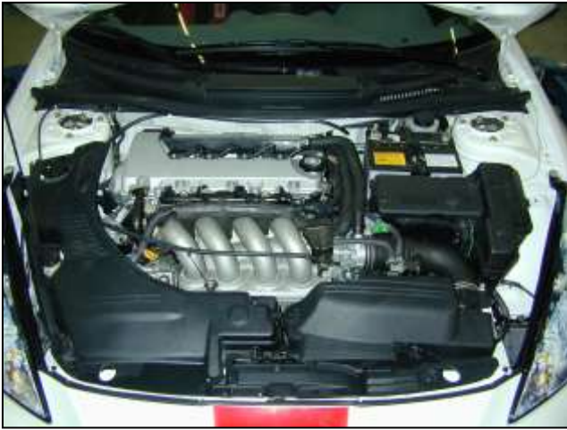
Stock air box system installed
