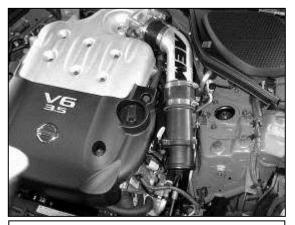
e. Place the 3" silicone coupler around the MAF sensor, not the AEM<sup>®</sup> MAF adaptor. Connect the assembly to the upper intake pipe. Use the #52 hose clamp around the throttle body and the #48 hose clamps for the 3" diameter tubing. Do not tighten the hose clamps.
