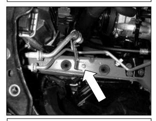
j. Remove the A/C line bracket bolt shown in the picture.
