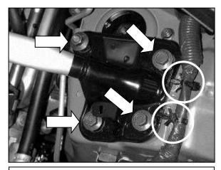
a. Remove the bolts holding the strut tower bar in place from both sides. Unclip the electrical wiring loom connections and remove the bar from the engine bay.
