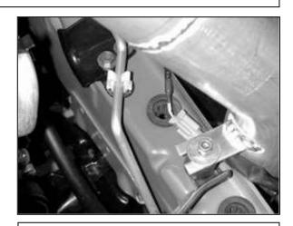
I. Line up the tab on the intake pipe with the rubber mount. Run the wheel speed sensor wire underneath intake pipe support tab. Make sure the plug and wire are not in a place where they will be pinched or damaged. Install the nut and washer according to the diagram below.
