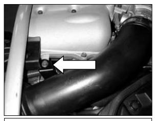
c. Remove the bolt securing the inlet pipe to the intake manifold.
