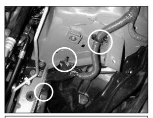
h. Unsnap the wiring loom fasteners from the inner fender.
