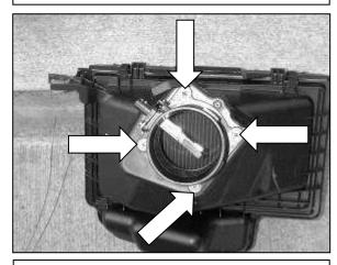
k. Remove the MAF sensor from the air filter assembly by removing the four mounting bolts.
