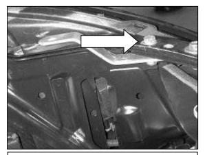
f. Install the 8mm bolt and washer included in the kit into the bolt hole exposed in step 2d. Attach the AEM<sup>®</sup> wiring harness bracket to the bolt on the underside and secure it in place with the included 8mm nylok nut.
