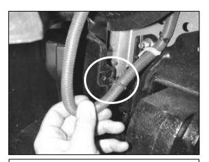
h. Inside the cavity behind the bumper, unsnap the wiring loom from the body.
