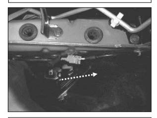
i. Looking where the factory air filter housing was, pull the wheel speed sensor plug shown in the picture from its mount. **NOTE: DO NOT unplug the sensor.**
