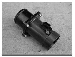
d. Using the four bolts and washers included in the kit, attach the  $\text{AEM}^{\textcircled{B}}$  MAF adaptor to the Nissan MAF sensor.
