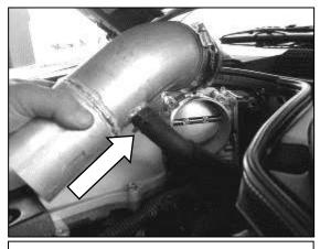
c. Attach the breather hose to the fitting to the AEM<sup>®</sup> upper intake pipe (the shorter one in the kit). Put the 3 ¼" to 3.0" silicone reducer on the end of the pipe closest to the bend. Place the 3 ¼" side of the silicone coupler over the throttle body. b. Install the rubber mount into the hole that was exposed when the A/C line bracket was removed to step 2j. Use the included spacer underneath the rubber mount to space it upward to clear the bracket. Tighten by hand.
