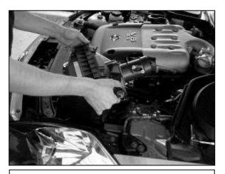
g. Gently pull directly upward on the air filter housing assembly until it unsnaps from its mounts. Remove it from the engine bay.
