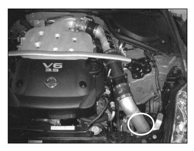
m. Position the intake pipe and air filter for the best fitment. Ensure that the intake system does not contact any part of the vehicle or any other components. Ensure the intake pipe does not come into contact with any of the adjacent A/C hard-lines. Contact may result in failure of the A/C system and costly repairs. After the intake system has been positioned correctly, tighten all hose clamps and the mounting tab hardware. Plug in the MAF sensor and re-install the strut-tower bar.
