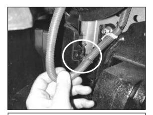
h. Inside the cavity behind the bumper, unsnap the wiring loom from the body.
