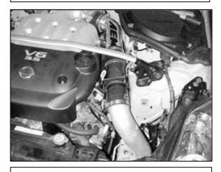
k. Install the 3" coupler and two #48 hose clamps on the end of the MAF adaptor. Insert the upper end of the lower intake pipe into the coupler.
