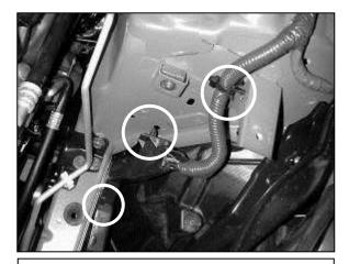
h. Unsnap the wiring loom fasteners from the inner fender.
