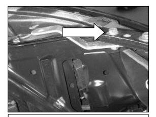
f. Install the 8mm bolt and washer included in the kit into the bolt hole exposed in step 2d. Attach the AEM® wiring harness bracket to the bolt on the underside and secure it in place with the included 8mm nylok nut.
