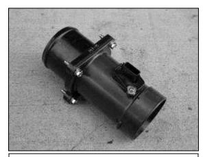
d. Using the four bolts and washers included in the kit, attach the AEM® MAF adaptor to the Nissan MAF sensor.
