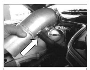
c. Attach the breather hose to the fitting to the AEM® upper intake pipe (the shorter one in the kit). Put the 3 ½" to 3.0" silicone reducer on the end of the pipe closest to the bend. Place the 3 ½" side of the silicone coupler over the throttle body.
