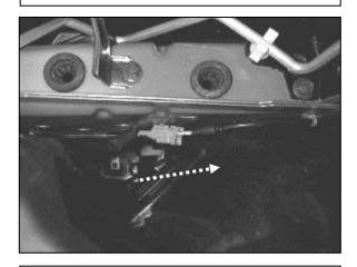
i. Looking where the factory air filter housing was, pull the wheel speed sensor plug shown in the picture from its mount.
