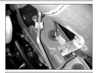
I. Line up the tab on the intake pipe with the rubber mount. Run the wheel speed sensor wire underneath intake pipe support tab. Make sure the plug and wire are not in a place where they will be pinched or damaged. Install the nut and washer according to the diagram below.
