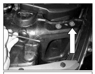
d. Pop out and remove the plastic fastener on the front air duct. Unsnap the duct and slide it forward. Remove the specified bolt as shown.
