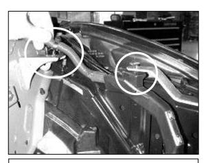
g. Snap the factory wiring harness into the bracket as shown. Insert the other plastic wiring loom holder into the hole from the bolt removed in step 2f of the previous section.
