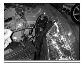
f. Remove the bolt holding the air filter housing assembly in place.
