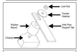
Proper installation of rubber mount assembly.
