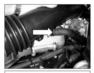
e. From the underside of the intake tube, detach the breather hose then remove the intake tube from the engine bay.
