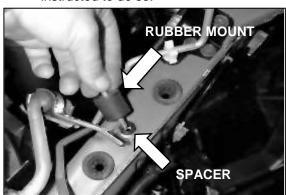
b. Install the rubber mount into the hole that was exposed when the A/C line bracket was removed to step 2j. Use the included spacer underneath the rubber mount to space it upward to clear the bracket. Tighten by hand.
