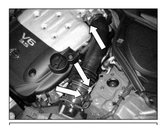
b. Loosen the hose clamps shown in the picture. Unplug the mass air flow (MAF) sensor and detach the MAF wiring harness from the sensor.
