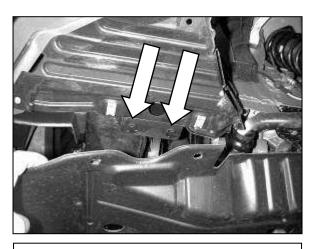
m. Pull down on the splash guard to reveal two plastic fasteners. Remove these fasteners.
