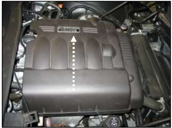
h. Remove the engine cover by pulling straight up on all four corners. This part will be reused.
