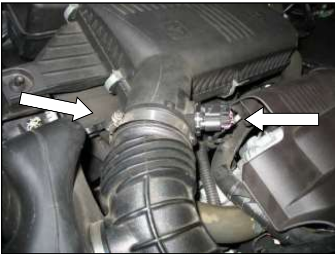
c. Loosen the hose clamp at the air box. Disconnect the mass air flow (MAF) sensor connector.
