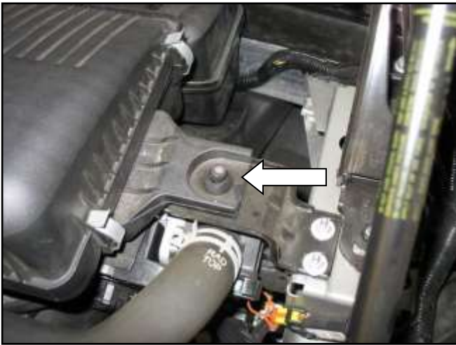
g. Loosen the remaining air box mounting bolt. Remove the air box from the engine bay, careful not to damage the hood.
