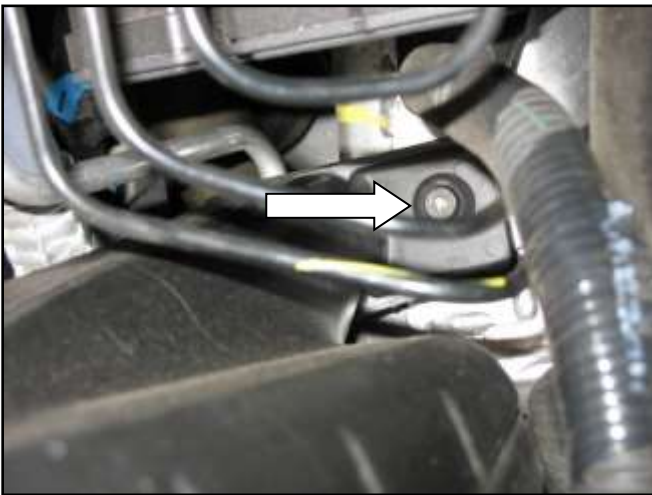
d. Loosen the inlet resonator tube mounting bolt located near the throttle body.
