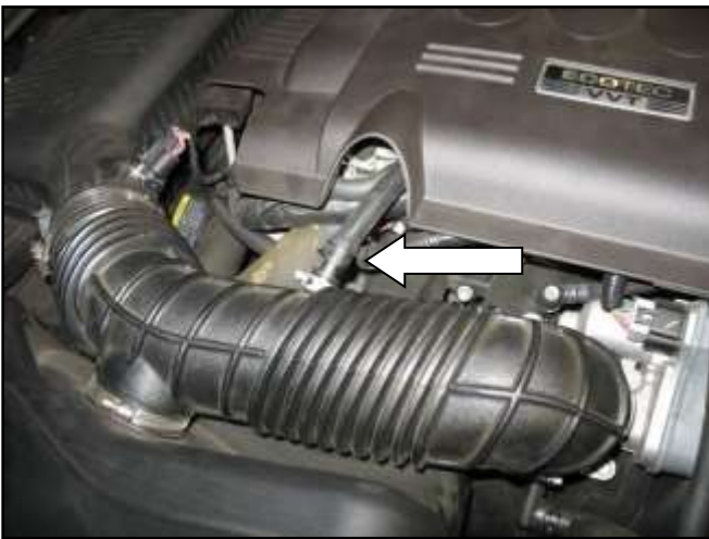
b. Unclasp the spring clamp. Remove the PCV breather hose from the inlet tube.
