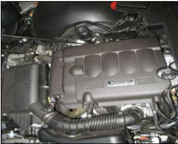
Factory air box system installed
