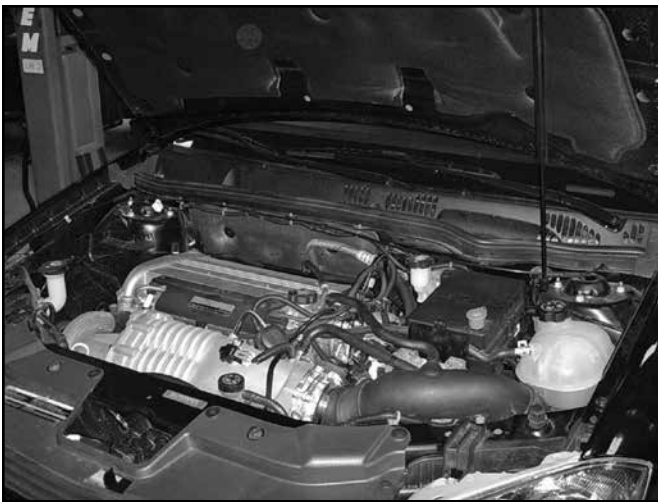
a. Factory air box system installed.
