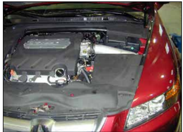
AEM® intake system installed
