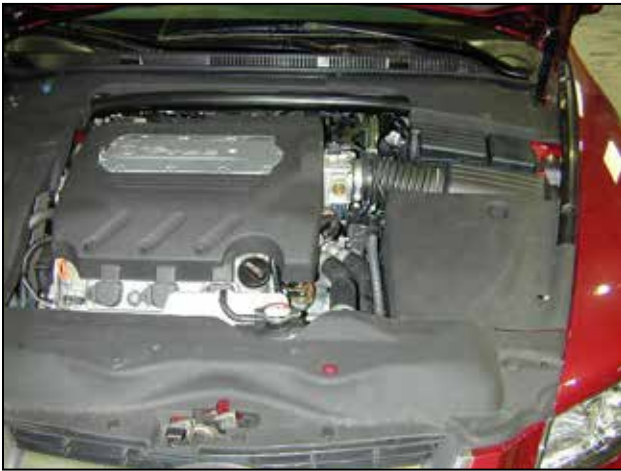
a. Factory air box system installed.
