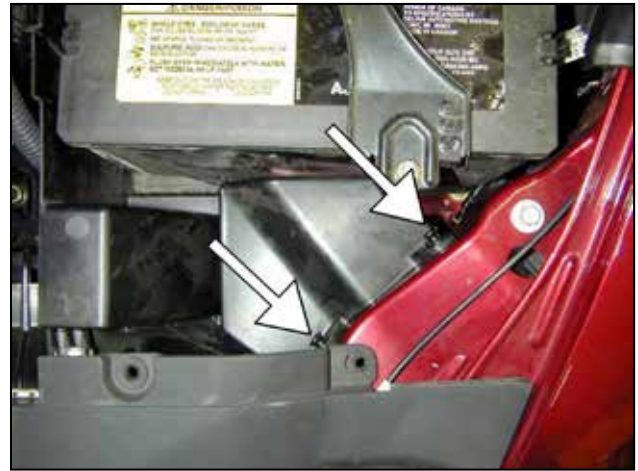
b. Remove plastic shrouding covering the battery. Remove the plastic air scoop in front of the battery by pulling out the two retaining clips and lifting scoop straight out.
