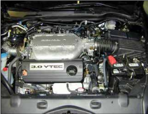
a. Factory air box system installed.
