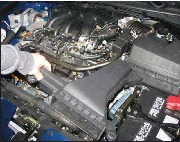
e. Remove the fresh air duct.
