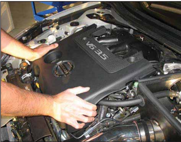
ah. Install the engine cover that was removed.
