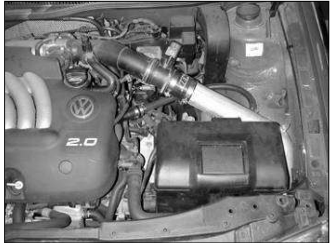
AEM® intake system installed
