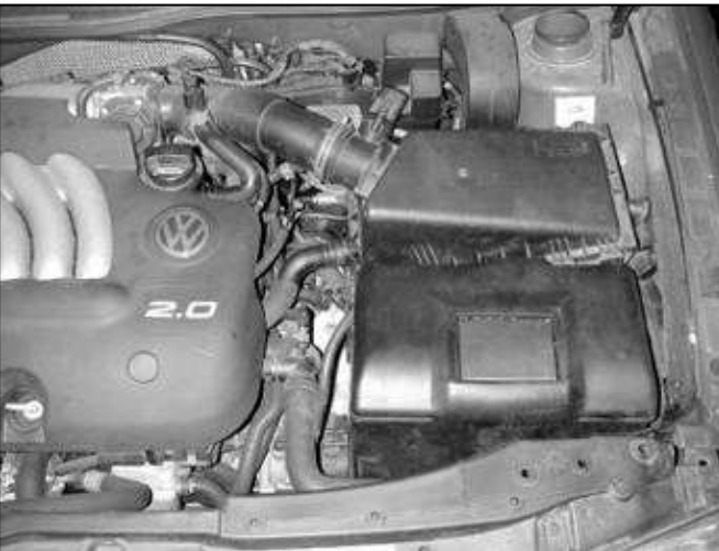
Factory airbox system installed
