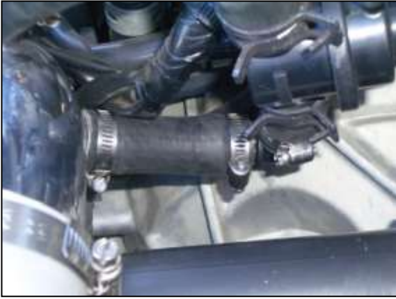
s. Attach the 4" end to the turbo intake pipe and secure with provided hose clamp.
