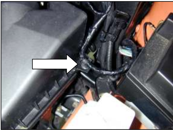
c. Unclip IAT and MAF sensor harness from the air box.
