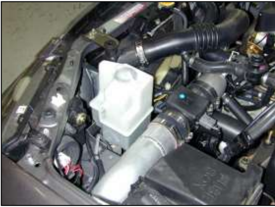
p. Attach the coolant overflow reservoir to the new bracket.
