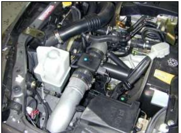
x. Reinsert the coolant reservoir on the new bracket.
