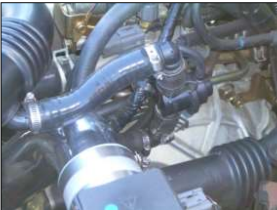
w. The BOV assembly should look like this.
