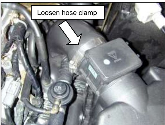
g. Loosen and remove hose clamp. Remove the air box assembly.
