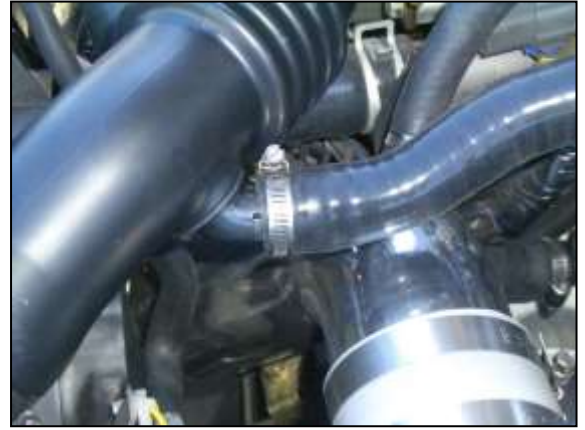
t. Attach the connector end to the BOV hose return side. Secure with hose clamp.
