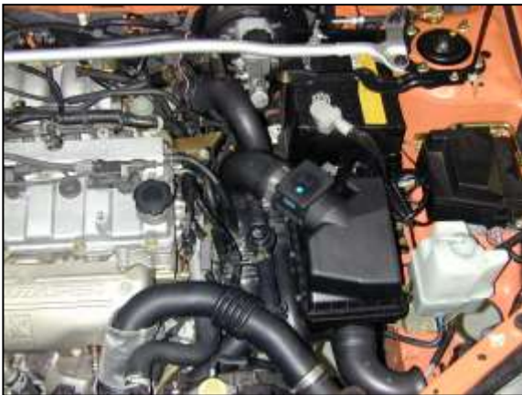
a. The stock air intake system.
