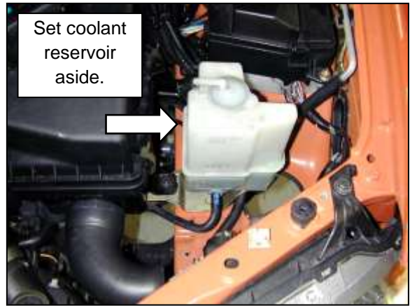
d. Remove the radiator fluid overflow bottle and set aside in the engine bay. Do not disconnect any of the coolant lines. There should be plenty of slack in the hose.
