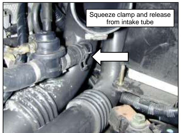
h. Squeeze clamp and release blow off valve hose from the specified intake tube.
