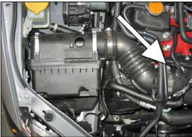
g. Loosen the hose clamp securing the factory air box inlet to the compressor inlet tube.
