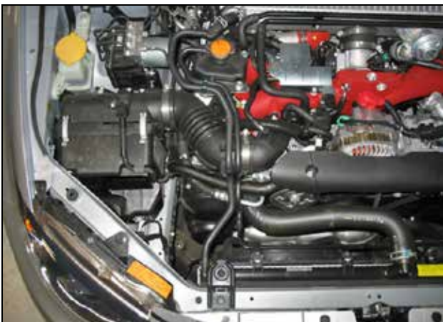
Factory air box system installed
