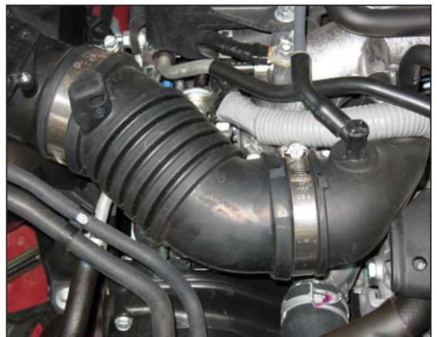
d. Loosen the two hose clamps on the stock air inlet tube and remove it.
