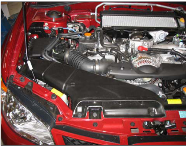
a. Stock air box system installed.
