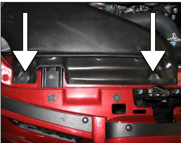
c. Remove the two mounting bolts securing the air inlet scoop and remove the scoop from the vehicle.
