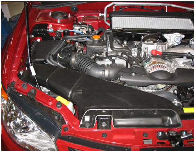
Stock air box system installed
