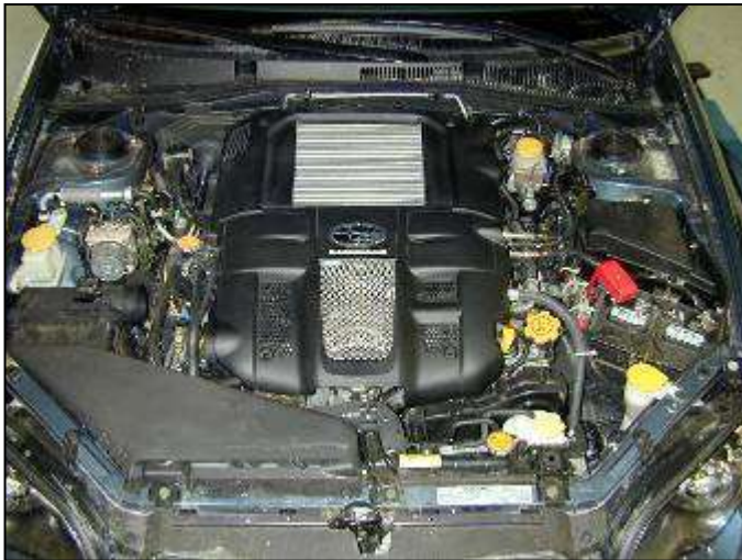
a. Factory air box system installed.
