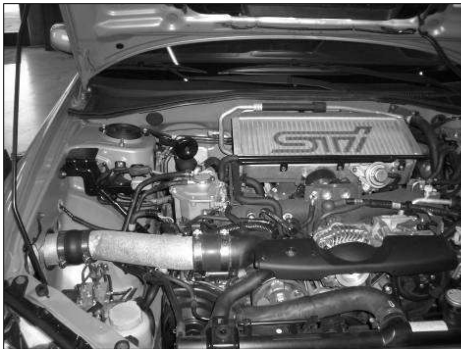
AEM® intake system installed.
