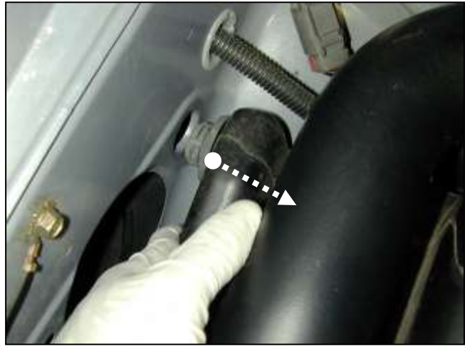
j. Gently pull the resonator from the fender. Remove the resonator and air box assembly.
