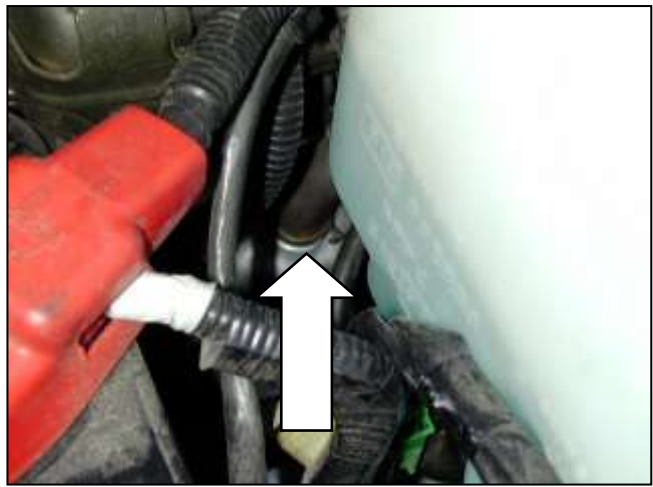
l. Remove the crankcase breather hose located on the driver's side.
