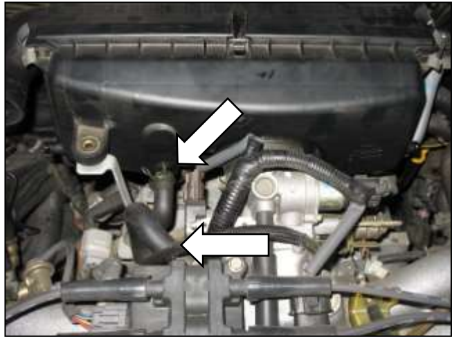
h. Remove the breather hose from the air box and manifold.
