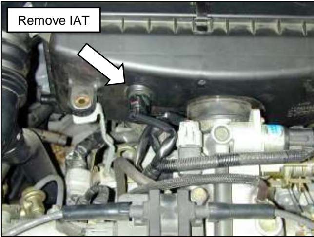
g. Remove the Inlet Air Temperature Sensor (IAT) from the air box. Be careful not to damage this sensor. Vehicles not equipped with IAT proceed to step h.
