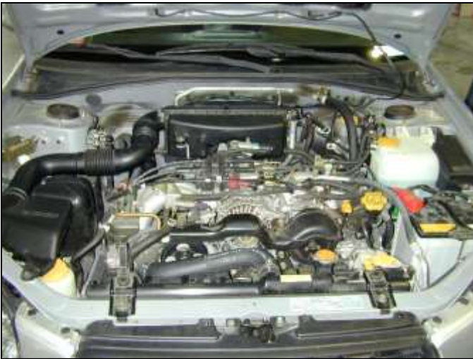
a. Factory air box system installed.
