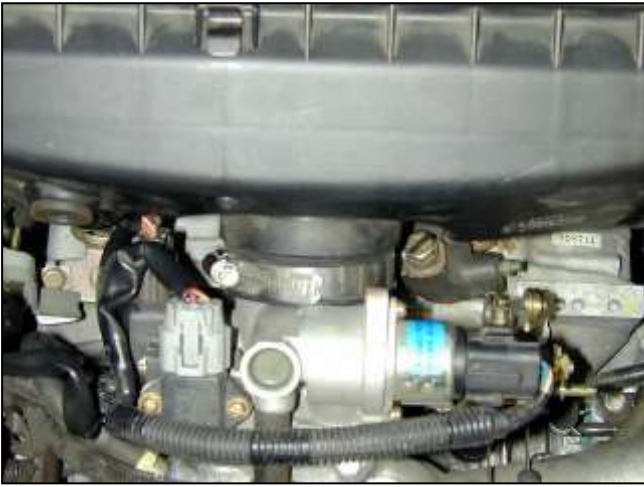
i. Loosen the hose clamp at the throttle body.
