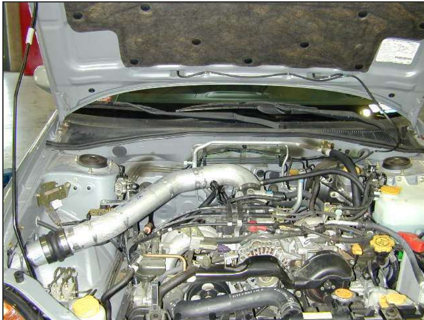
AEM ® intake system installed
