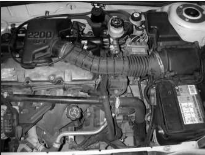
a. Factory air box system installed.
