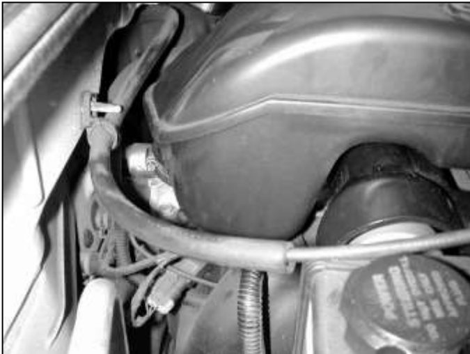
e. Loosen the hose clamp at the throttle body.
