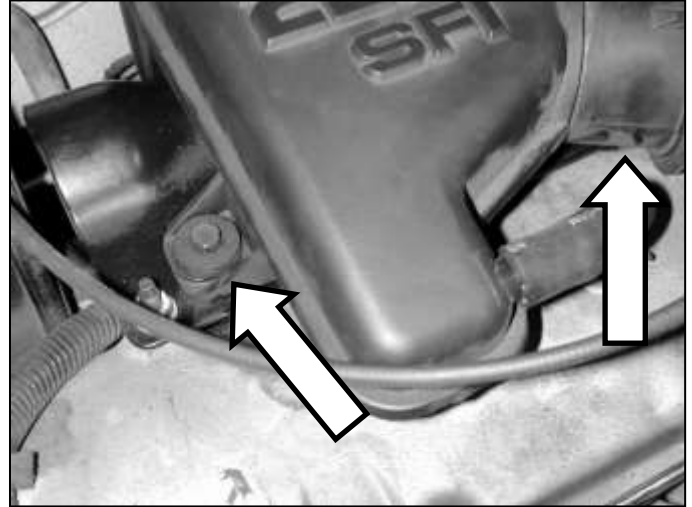
d. Remove bolt. Release the breather hose from the valve cover.
