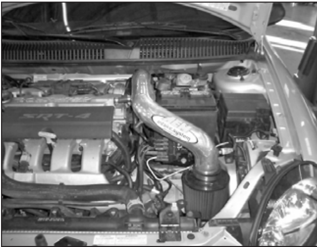
a. Dodge Neon SRT-4 with AEM® intake system (Part# 22-425) installed.
