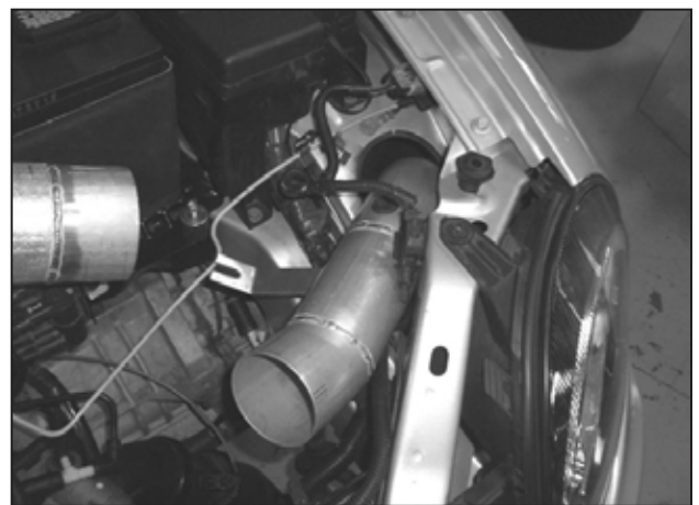
s. Insert the lower intake tube into the fender well cavity as shown.
