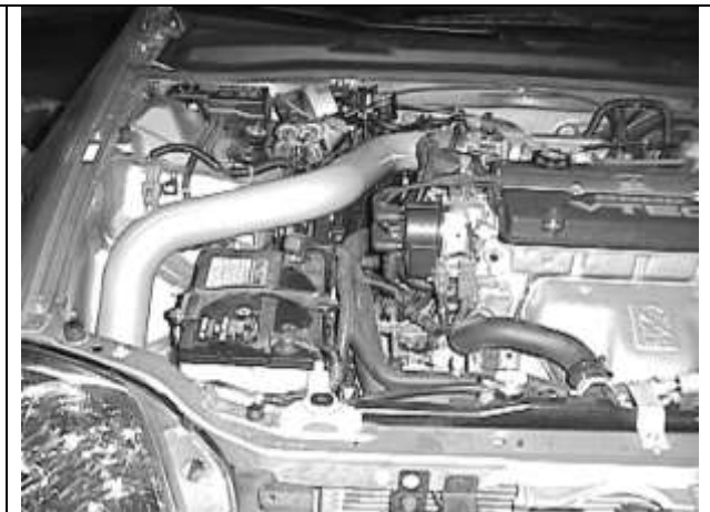
Fig 8: Intake tube installed
