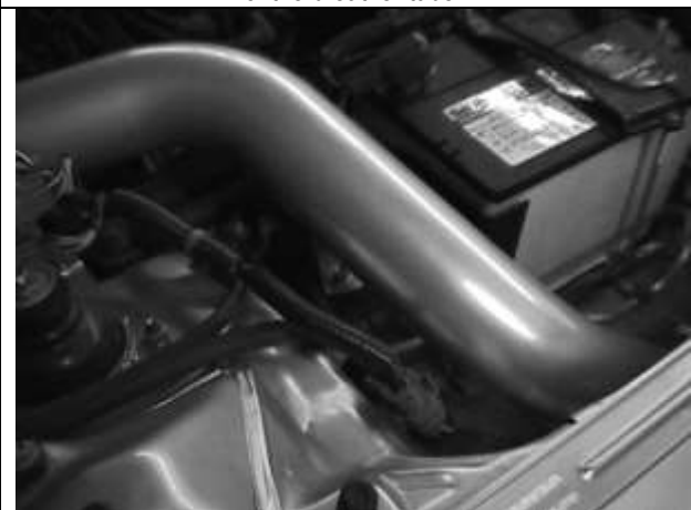
Fig 11: Intake pipe installed. Note mounting bolt.
