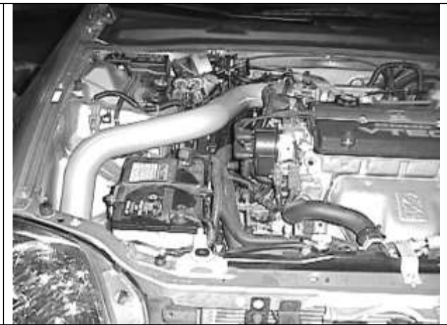
Fig 8: Intake tube installed
