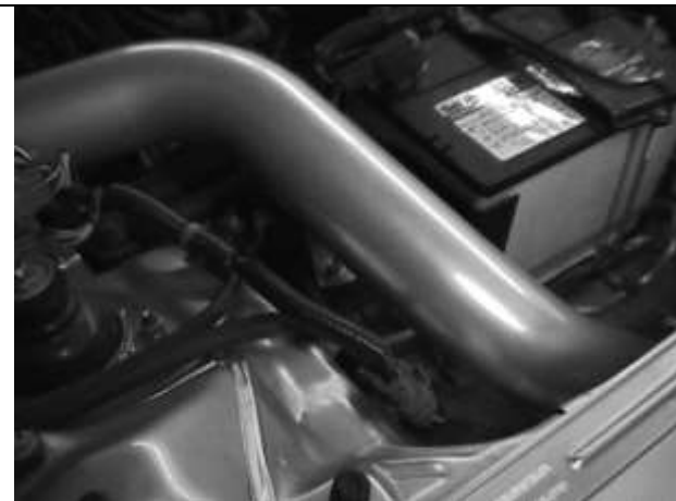
Fig 11: Intake pipe installed. Note mounting bolt.
