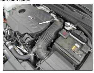
2. Release the spring clamps and then disconnect the vent lines and BOV hose.
