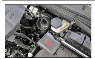
7. Install the provided coupler (5-1067) onto the turbo inlet and secure with the provided hose clamp.
