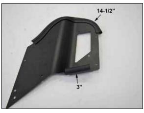
11. Cut the remaining edge trim into lengths of 3" and 14-1/2" and then install onto the heat shield lid as shown.
