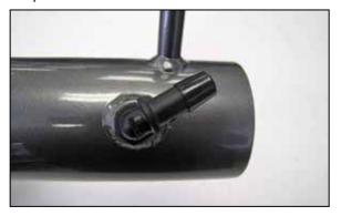
8. Install the  $90^{\circ}$  vent fitting onto the AEM $^{\circ}$  intake tube as shown.
