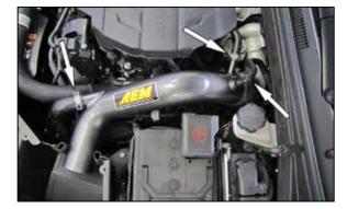
10. Install the vent lines and BOV hose onto the AEM® intake tube and secure with the factory spring clamps.
