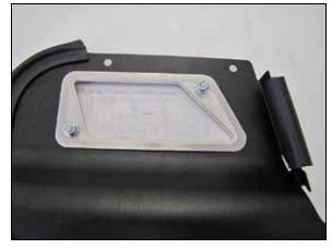
12. Install the AEM® window into the heat shield lid with the spacer between the lid and window and secure with the provided hardware.
