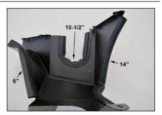
5. Cut the provided edge trim into sections of 6",10-1/2", 14" from the 35" and then install it onto the heat shield as shown.
