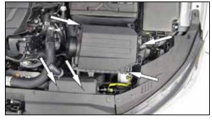
4. Remove the two push pins that secure the fresh air intake duct. Remove the three bolts that secure the factory air filter housing and then remove the housing from the vehicle.
