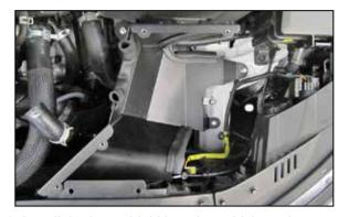
6. Install the heat shield into the vehicle and secure with the provided hardware.
