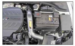
9. Install the intake tube into the coupler at the turbo and secure with the provided hose clamp.
