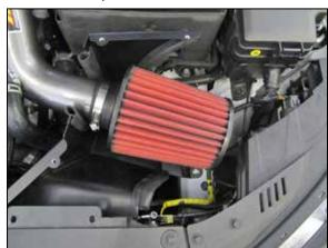
13. Install the AEM® air filter onto the intake tube and secure with the provided hose clamp.
