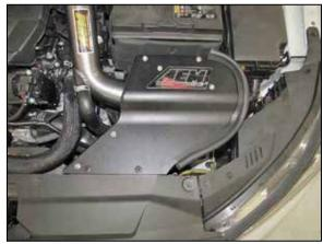
14. Install the heat shield lid and secure with the provided hardware.
