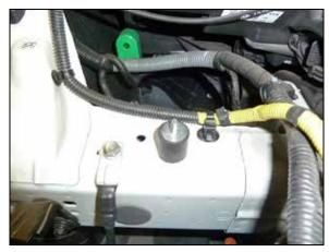
10. Install the provided rubber mounted stud into the air filter housing mounting location on the frame rail as shown
