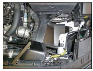
11. Install the heat shield into the vehicle and secure with the hardware provided.
