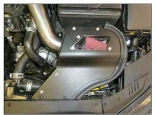
18. Install the heat shield lid and secure with the provided hardware.
