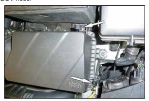
5. Release the two spring clamps that secure the upper air filter housing and then remove the upper housing and intake hose from the vehicle.
