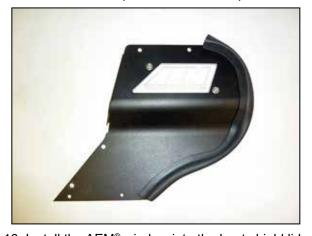
16. Install the AEM® window into the heat shield lid and secure with the provided hardware. Install the long edge trim onto the heat shield lid.
