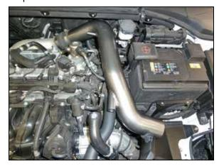
13. Install the intake tube into the coupler and onto the heat shield, adjust for best fit and then secure with the provided hardware.
