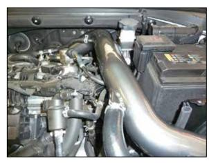
14. Connect the PCV hose and BOV hose to the AEM® intake tube and secure with the factory spring clamps.
