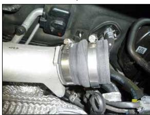
12. Install the provided coupler (08439) onto the turbo inlet and secure with the provided hose clamp.
