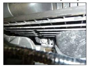
8. Remove the front air filter housing mounting bolt and remove the lower air filter housing from the vehicle. It may be necessary to move or remove the battery hold down to gain access to the bolt.
