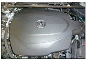
2. Lift the engine cover and remove it from the engine.
