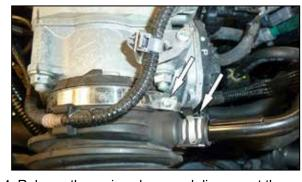
4. Release the spring clamp and disconnect the crank case vent line from the factory intake tube. Loosen the hose clamp that secures the factory intake tube to the throttle body.
