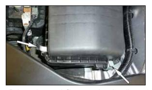
5. Release the two air filter upper housing clips and remove the upper housing, intake tube and air filter from the vehicle.
