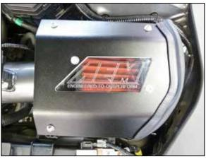
21. Install the cover assembly onto the heat shield and secure with the provided hardware.
