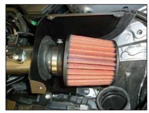
18. Install the AEM® air filter and secure with the provided hose clamp.
