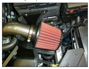
12. Install the AEM® air filter and secure with the provided hose clamp.
