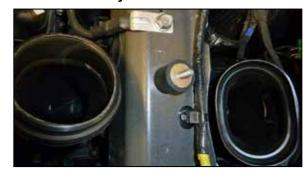
6. Install the provided rubber mounted stud onto the frame rail as shown.
