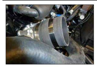
7. Install the provided coupler (#08421) onto the throttle body and secure with the provided hose clamp.
