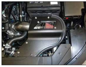
15. Install the lid onto the heat shield and secure with the provided hardware.
