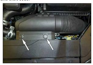
2. Remove the two push pins that secure the fresh air intake duct and then remove the fresh air intake duct from the vehicle.
