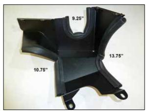
9. Install the three sections of edge trim onto the heat shield as shown.
