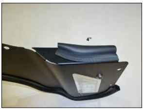
14. Install the remaining edge trim onto the heat shield as shown.
