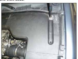
2. Remove the pins that secure the drivers side rear decorative engine cover and then remove the cover.
