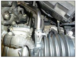
5. Disconnect the crank case vent tube from the factory intake boot.
