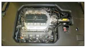
19. Reinstall the decorative engine covers and reconnect the negative battery cable.
