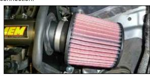
18. Install the AEM® air filter onto the intake tube and secure with the provided hose clamp.
