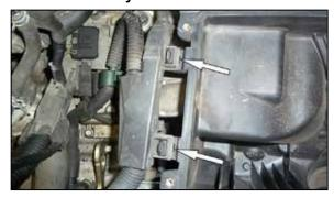
8. Unclip the wiring harness from the lower air filter housing.
