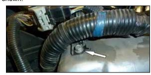
13. Remove the wiring harness mounting bolt shown on the shock tower.
