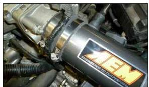
16. Install the AEM® intake tube into the heat shield and then into the coupler, adjust the tube for best fit and secure with the provided hardware.
