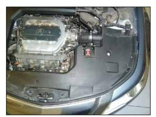
3. Remove the clips that secure the drivers side front decorative cover and then remove the cover.
