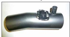
10. Remove the mass air sensor from factory air filter housing and then install into the AEM® intake tube and secure with the provided hardware. Install the crank case vent adapter grommet into the AEM® intake tube as shown.
