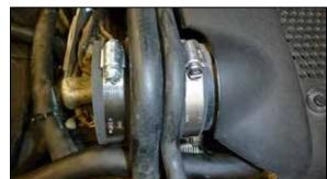
12. Install the provided coupler (5-275) onto the inlet tube and secure with the provided hose clamp.
