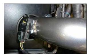
16. Reconnect the mass air sensor electrical connection and secure the wiring harness with the provided tie wrap to the bracket on the intake tube.
