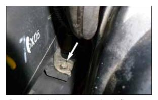
5. Remove the bolt that secures the air filter housing to the frame rail.
