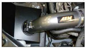
13. Install the intake kit into the vehicle so the intake tube goes into the coupler hose and the studs on the inner fender protrude through the holes in the heat shield.
