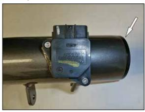
10. Remove the mass air sensor from the factory air filter housing and install it into the AEM intake tube and secure with the provided hardware. Install the provided venturi sleeve into the intake tube so that the slot goes around the mass air sensor.
