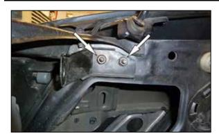
7. Remove the two nuts that secure the filter housing mounting bracket to the inner fender and then remove the mounting bracket from the vehicle.
