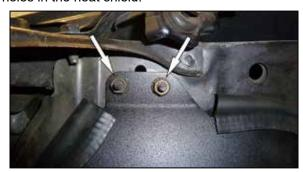
14. Secure the heat shield to the inner fender using the factory nuts removed earlier.
