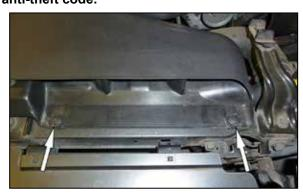
2. Remove the two plastic retaining clips that secure the fresh air intake duct.
