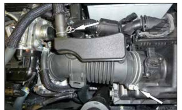
5. Remove the PCV hose from the factory intake tube and then loosen the hose clamp that secures the intake hose to the air filter housing and then remove it from the vehicle.
