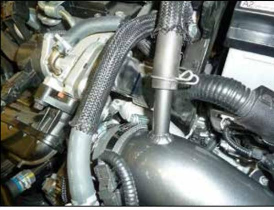
22. Connect the PCV hose to the AEM® intake tube and secure with the factory spring clamp.
