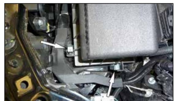
6. Release the two clips that secure the upper air filter housing and then remove the upper housing from the vehicle.
