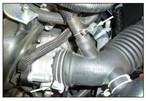
4. Release the clamp and disconnect the crank case vent hose from the intake hose. Loosen the hose clamp that secures the intake hose to the throttle body and then disconnect the hose from the throttle body.
