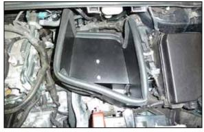
13. Set the heat shield onto the mounting brackets and around the fresh air intake and then secure with the provided hardware.
