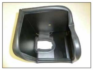
12.Install the two remaining edge trims onto the heat shield as shown.
