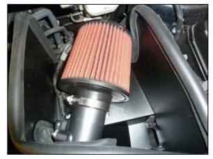
20. Install the air filter onto the intake tube and secure with the provided hose clamp. Adjust the intake tube for best fit and then secure with the provided hose clamps.
