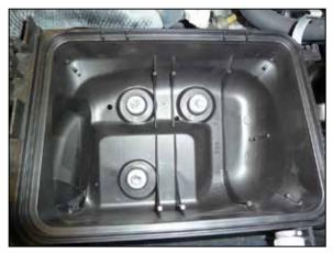
7. Remove the three bolts that secure the lower air filter housing and then remove the lower housing from the fresh air intake and vehicle. NOTE: AEM recommends that customers do not discard factory air intake.
