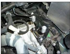
9. Install the heat shield mounting grommets as shown onto the factory air filter housing mounting location using the provided hardware.
