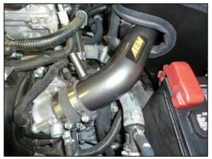
17. Install the intake tube through the heat shield and into the coupler at the throttle body. Do not tighten at this time.
