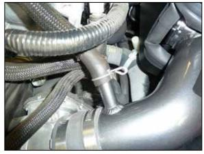
18. Connect the crank case vent to the AEM® intake tube and secure with the factory clamp.
