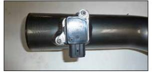
15. Remove the mass air sensor from the factory air filter housing and install it into the AEM® intake tube using the provided hardware.
