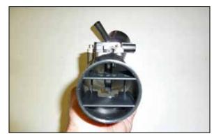
16. Using a small amount of the provided superglue on the lip of the air straightener insert, install the air straightener into the tube as shown. NOTE: install the so the blades are perpendicular to the sensor as shown.
