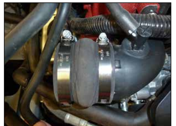
16. Install the provided hump coupler (08185) onto the turbo inlet and secure with the provided hose clamp.
