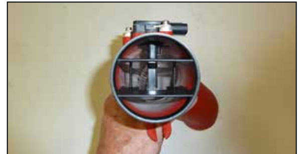
13. Place three small drops of the provided glue next to the lip of the maf sleeve and then install the maf sleeve so that the blades are perpendicular to the maf as shown.
