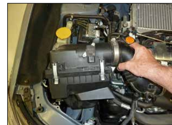
6. Remove the bolt that secures air filter housing to the frame rail and then remove the air filter assembly from the vehicle.
