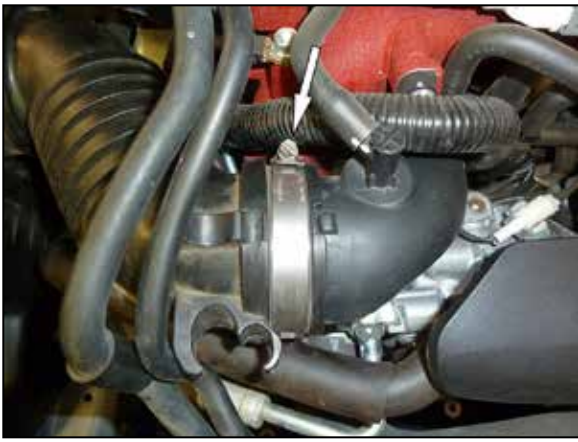
4. Loosen the hose clamp that secures the intake hose to the turbo inlet.
