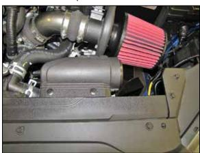
13. Remove the hose from the fresh air intake duct and then reinstall the duct and secure with the factory retaining pins.
