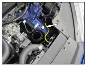
4. Install the rubber mounted stud into the frame rail at the air filter housing mounting location.
