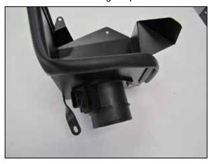
8. Remove the mass air sensor from the factory air filter housing and install it into the AEM® heat shield and secure with the provided hardware.
