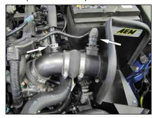
11. Reconnect the mass air sensor electrical connection. Connect the crank case vent hose and secure with the factory spring clamp.
