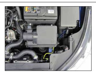
3. Remove the fresh air intake duct from the vehicle. Remove the three bolts that secure the air filter housing and then remove the air filter housing from the vehicle.
