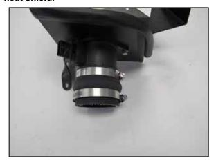
9. Install the hump coupler (08185) onto the mass air sensor and secure with the provided hose clamp.
