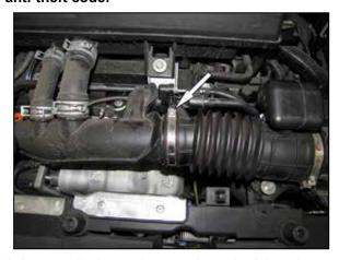
2. Loosen the hose clamp at the turbo inlet tube.
