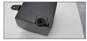
6. Remove the mounting grommet from the factory air filter housing and install it into the AEM® heat shield as shown.
