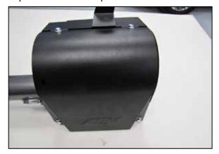
8. Install the heat shield lid onto the heat shield and secure with the provided hardware.
