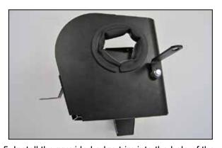
5. Install the provided edge trim into the hole of the heat shield as shown. Install the mounting bracket (010051A) onto the heat shield and secure with the provided hardware.
