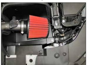
13. Install the AEM® air filter and secure with the provided hose clamp.
