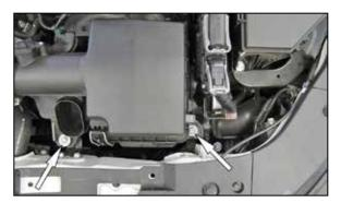
5. Remove the two bolts that secure the air filter housing and then lift up the intake assembly to remove it from the vehicle.
