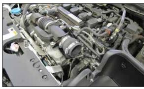
11. Install the provided hump coupler (08487) onto the turbo inlet and secure with the provided hose clamp.
