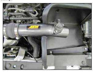
12. Install the AEM® intake tube into the coupler at the turbo inlet and then align the mounting stud with the hole in heat shield. Adjust the intake tube for best fit and then secure with the provided hardware and hose clamp.
