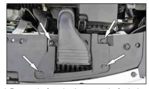
4. Remove the four pins that secure the fresh air intake to the core support.
