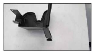
7. Remove the mounting grommet from the factory air filter housing and install it into the AEM® heat shield as shown.
