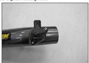
10. Remove the mass air sensor from the factory intake tube and install it into the AEM® intake tube and secure with the provided hardware.
