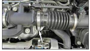
3. Loosen the hose clamp that secures the intake tube to the turbo inlet pipe.
