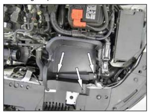
9. Install the heat shield assembly into the vehicle and secure with the provided hardware and one of the push pins that originally secured the fresh air intake. Install the three remaining push pins to fill the original mounting holes.
