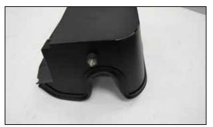
8. Install the rubber mounted stud onto the heat shield using the provided hardware.
