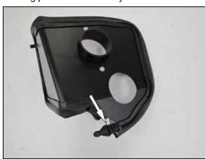
12. Install the mounting post from the previous step onto the AEM® heat shield as shown.
