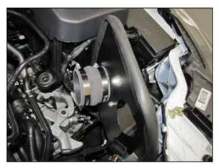
14. Install the provided coupler hose (087121) onto the filter adapter and secure with the provided hose clamp.
