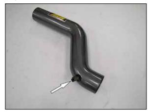
15. Install the grommet provided and the factory inlet air temperature sensor into the AEM® intake tube as shown.
