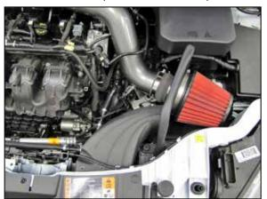
20. Install the AEM® fresh air duct onto the core support and into the AEM® heat shield.
