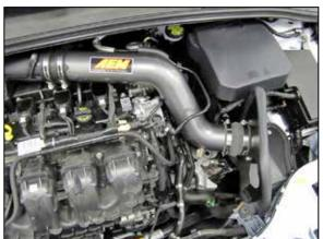
17. Install the AEM® intake tube into the factory coupler and then into the AEM® coupler, adjust the tube for best fit and then secure with the provided hose clamps.
