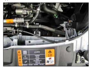
21. Using the Fresh air duct as a guide, mark the two hole locations onto the fresh air duct in the core support. Next remove the AEM® fresh air duct and drill two ¼"id holes into the factory fresh air duct at the marked locations.
