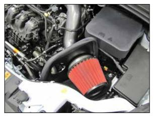
19. Install the AEM® air filter onto the filter adapter and secure with the provided hose clamp.
