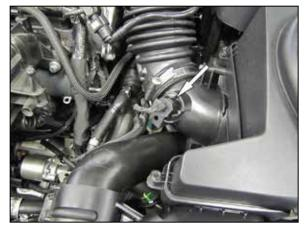
4. Disconnect the inlet air temperature sensor electrical connection.
