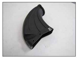
23. Install the two clips from the previous step onto the AEM® fresh air duct in the same position as the factory.
