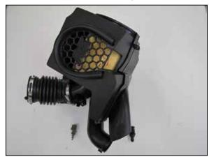
11. Remove the inlet air temperature sensor and mounting post from the factory air box.
