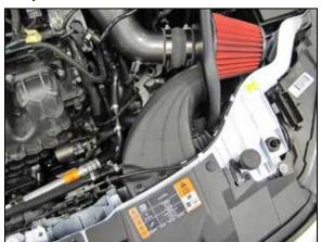
24. Install the AEM® fresh air duct into the heat shield and core support as shown and secure with the two provided retaining clips.
