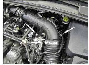
3. Remove the bolt securing the factory intake tube to the engine shown. Next loosen the hose clamps and unhook the vent line from the intake tube and remove the intake tube from the vehicle.
