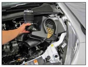
6. Lift and dislodge the air box from its mounting grommets and then remove the air box from the vehicle.
