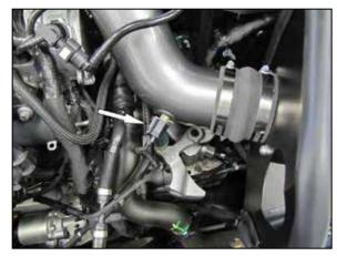
18. Reconnect the inlet air temperature sensor electrical connection.
