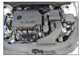
2. Lift off the decorative engine cover. Remove the fresh air intake duct from the factory air filter housing and core support.
