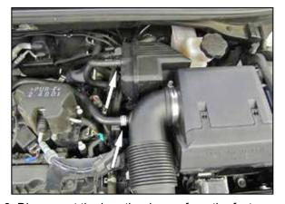
3. Disconnect the breather hoses from the factory intake tube and intake plenum.
