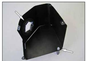
8. Install the provided mounting stud onto the heat shield as shown. Install the provided edge trim into the hole of the heat shield as shown.
