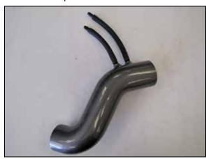
10. Install the provided vent lines and fittings onto the AEM® intake tube as shown.
