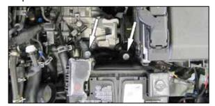
7. Install the two-provided rubber mounted studs into the factory air filter housing mounting locations.
