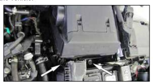
5. Remove the two bolts that secure the factory air filter housing and then remove the factory housing from the vehicle.
