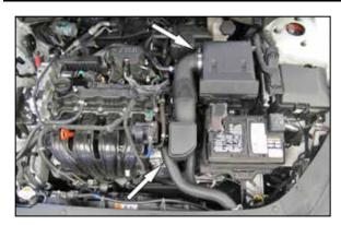
4. Loosen the hose clamps that secure the factory intake tube and then remove the intake tube from the vehicle.
