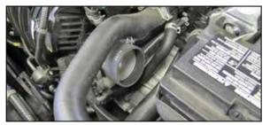
6. Install the provided coupler hose (08711) onto the throttle body and secure with the provided hose clamp.
