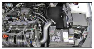
11.Install the AEM® intake tube into the heat shield and into the coupler at the throttle body, adjust the tube for best fit and then secure with the provided hose clamp.
