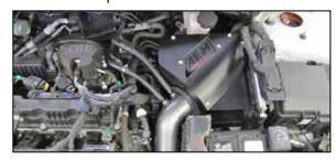
15. Connect the factory vent lines to the lines installed onto the AEM® intake tube.
