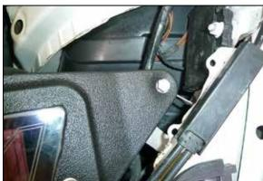
12. Install the remaining spacer into the air filter housing and then secure the housing with the provided hardware.
