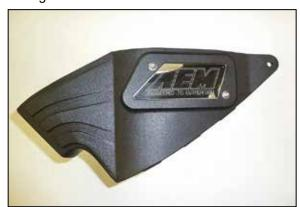
8. Install the AEM® badge into the filter housing and secure with the provided hardware.
