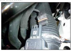
2. Disconnect the mass air sensor electrical connection. Loosen the hose clamp that secures the factory intake tube to the air filter housing.
