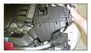
5. Remove the factory air filter housing from the vehicle.
