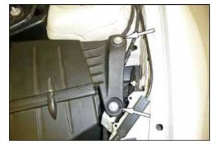
4. Remove the two bolts shown that secure the factory air filter housing to the inner fender.
