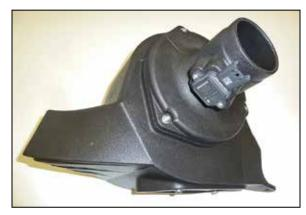
10. Install the AEM® mass air housing onto the filter housing and secure with the provided hardware.
