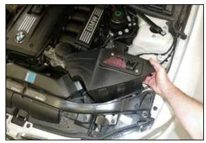
11. Install the AEM® filter housing assembly into the vehicle so that it sits on the factory bushings and the fresh air duct installs onto the AEM® air filter housing.
