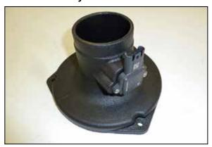
6. Remove the mass air sensor from the factory housing and install it into the AEM® housing and secure with the provided hardware.
