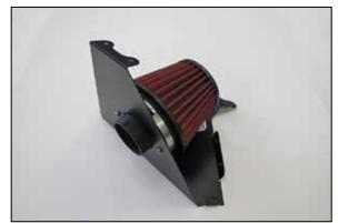
7. Install the provided filter adapter into the heat shield and secure with the provided hardware. Install the provided air filter onto the filter adapter and secure with the provided hose clamp.
