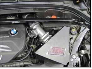
11. Install the provided coupler onto the intake tube but do not secure. Install the intake tube assembly into the factory intake hose and align with the filter adapter, slide the coupler onto the adapter and adjust the assembly for best fit. Secure the intake tube assembly with the provided hose clamps. Reconnect the mass air sensor electrical
