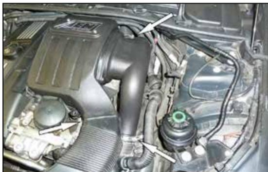
15. Install the AEM® intake assembly onto the factory mounting pins, then align and connect the fresh air intake duct. Connect the factory intake tubes to the AEM® housing and then secure with the factory hose clamps.
