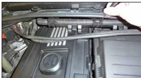
3. Remove the wiring from the lower guide and then unclip the three lower guide retaining clips and remove the lower guide from the vehicle.
