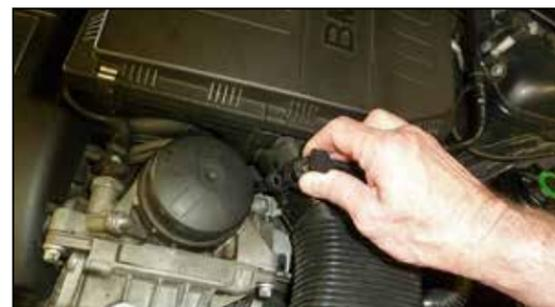
5. Squeeze the sides of the vacuum breather hose connection and disconnect.
