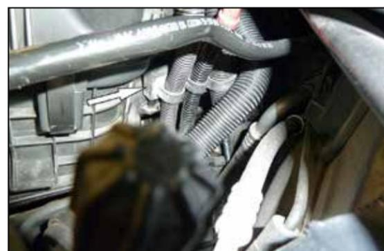
6. Remove the rubber wiring harness mounts from the rear of the air filter housing by pulling up to disengage.
