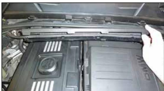
2. Unclip the four wiring harness guide retaining clips and then remove the upper wiring harness guide.
