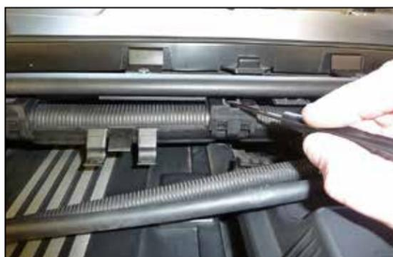
4. Unclip the rear wiring harness to release and then pull the harness forward.
