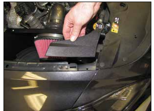
16. Lift up the plastic corner trim and remove for access to the heat shield lid.
