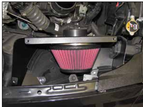
12. Install the heat shield assembly into the vehicle and secure with the provided hardware.
