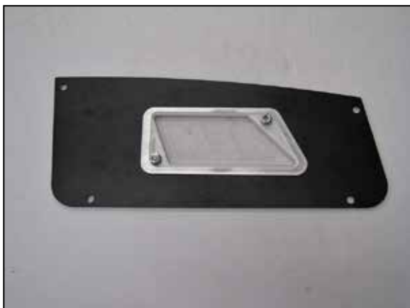
7. Install the AEM® logo window into the heat shield lid and secure with the provided hardware.
