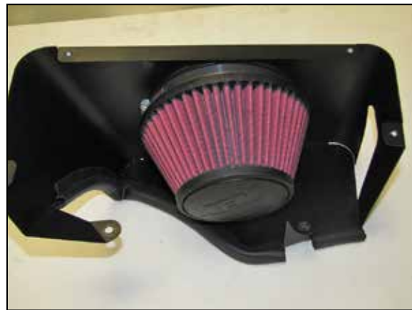
11. Install the AEM® air filter and secure with the provided hose clamp.
