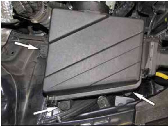
5. Remove the plastic housing and then remove the housing from the vehicle.
