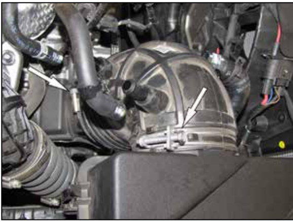
4. Loosen the hose clamps that secure the factory intake hose and remove the hose from the vehicle.
