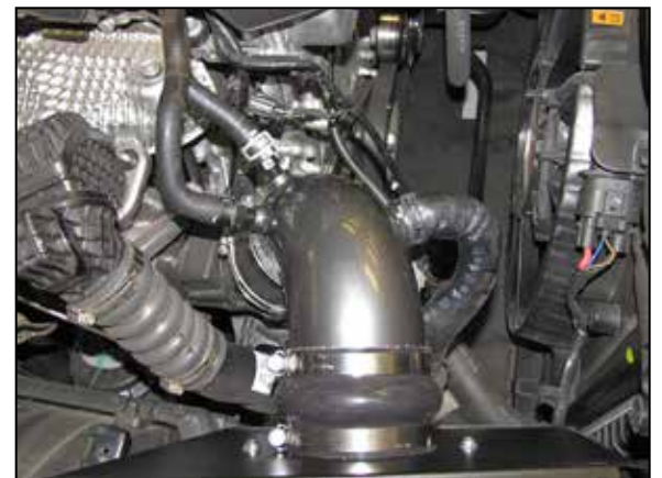
15. Install the AEM® intake tube into the couplers and secure with the provided hardware. Connect the vent lines and BOV hose and secure with the factory spring clamps.
