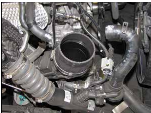
6. Install the provided step coupler onto the turbo inlet plenum and secure with the provided hose clamp.
