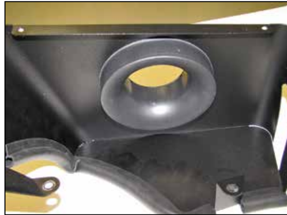
10. Install the heat shield assembly into the vehicle shield and secure with the provided hardware.
