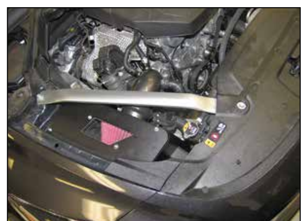
18. Reinstall the strut tower brace and secure with the factory hardware.
