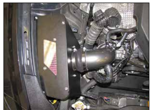
17. Install the heat shield lid and secure with the provided hardware then reinstall the plastic corner trim.
