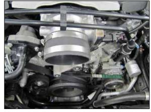
18. Install the provided coupler (08761) onto the throttle body and secure with the provided hose clamps.
