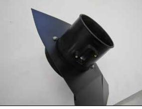
13. Install the provided mass air sensor housing into the provided heat shield and secure with the hardware provided.
