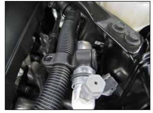
8. Disconnect the sound tube from the A/C line.
