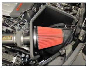
24. Install the AEM<sup>®</sup> air filter and secure with the provided hose clamp.
