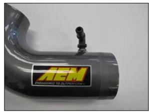
20. Install the 90° vent fitting into the AEM® intake tube as shown.
