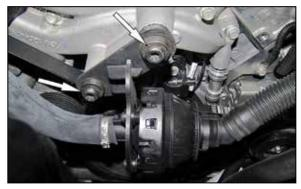
6. Remove the two bolts that secure the sound drum to the engine.
