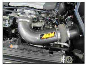
21. Install the AEM® intake tube into the hump coupler and then into the coupler at the throttle body, adjust the tube for best fit and then secure with the provided hose clamps.
