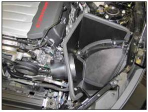
17. Install the heat shield assembly into the vehicle so the mounting studs engage the factory grommets.
