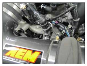
22. Connect the factory crank case vent line to the quick connect fitting installed into the AEM<sup>®</sup> intake tube.
