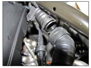
9. Disconnect the sound tube quick disconnect and then remove the complete sound tube assembly.
