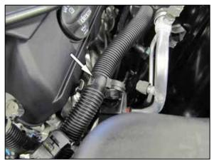
7. Open the clamp that secures the sound tube to the factory air filter housing.
