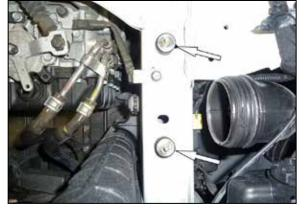
8. Install the two-provided rubber mounted studs onto the frame as shown.
