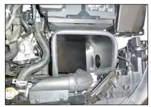
9. Install the heat shield into the vehicle so the so that the studs protrude though holes in the heat shield, secure the heat shield with the provided hardware.
