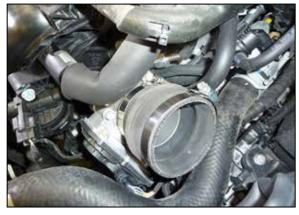
10. Install the provided coupler (08421) onto the throttle body and secure with the provided hose clamp.
