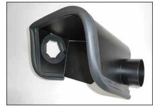
7. Install the 12" edge trim into the hole of the heat shield and the 34" section around the outside of the heat shield as shown.
