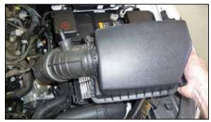
4. Loosen the hose clamp that secures the intake tube to the throttle body, release the two clips that secure the upper air filter housing and then remove the upper air filter housing and intake tube assembly. 5. Remove the three bolts that secure the lower air filter housing to the inner fender and then remove the lower air filter housing from the vehicle. **NOTE: AEM recommends that customers do not discard factory air intake.**
