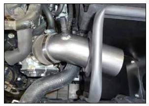
12. Install the AEM<sup>®</sup> tube through the heat shield and then into the coupler at the throttle body. Do not secure at this time.
