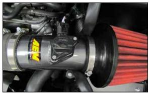
15. Reconnect the mass air sensor electrical connection.
