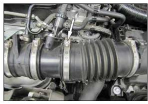
3. Loosen the hose that secures the intake hose to the turbo inlet pipe.
