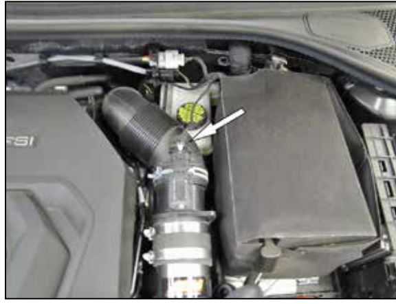
20. Reconnect the mass air sensor electrical connection.
