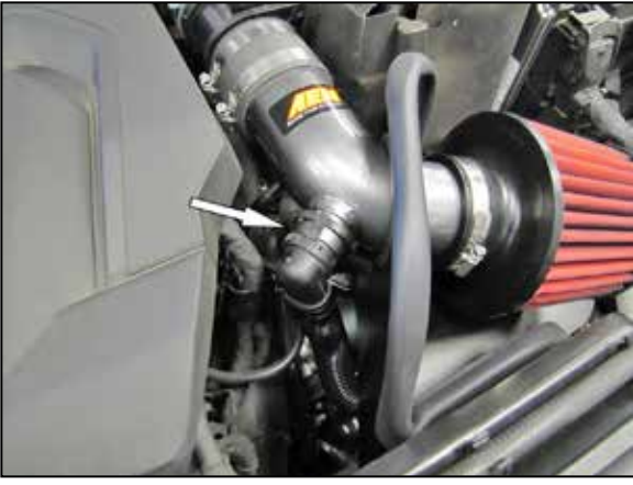
19. Connect the air injection hose to the AEM® intake tube.
