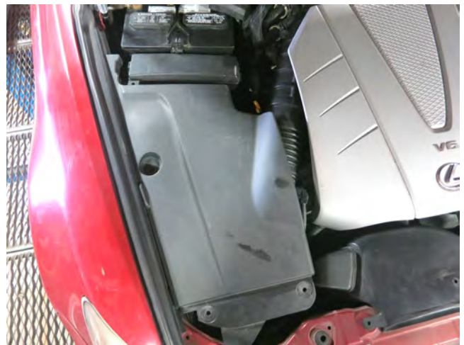
b. Remove the plastic shrouding to the side of the engine by removing the clip and pulling it out.
