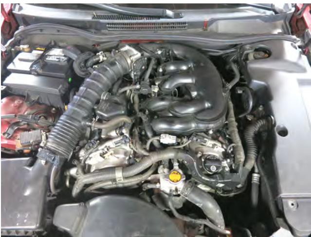
c. Remove the engine cover by pulling up gently to release it from its rubber grommets.
