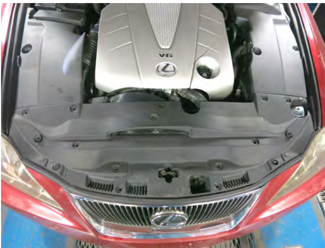
a. Remove the front apron by removing the plastic push rivets and lifting it out of the engine bay.
