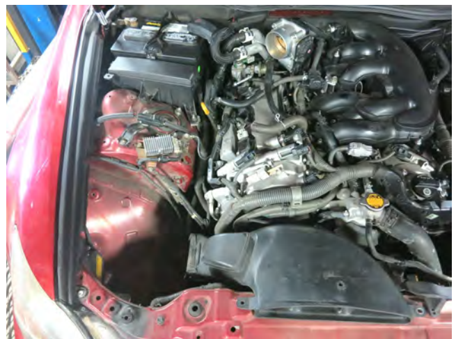
j. Lift the air box base up and out of the engine bay. Do not remove the air scoop.
