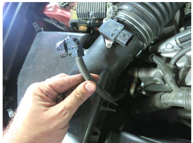
d. Disconnect the Mass Air Flow (MAF) sensor harness from the MAF sensor and air box.
