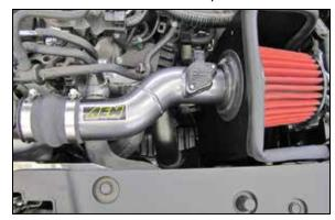
11. Install the AEM<sup>®</sup> intake tube through the heat shield and into the AEM<sup>®</sup> air filter, then install onto the turbo inlet. Align the tube for best fit and then secure with the provided hose clamp.
