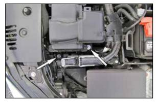
4. Remove the two bolts that secure the air filter housing to the vehicle. **NOTE: AEM recommends that customers do**
