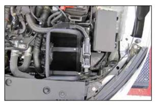
7. Install the heat shield assembly onto the frame rail and secure with the provided hardware. **NOTE: The heat shield will bolt to the rubber mounted stud and to the factory rear air filter housing mounting location.**
