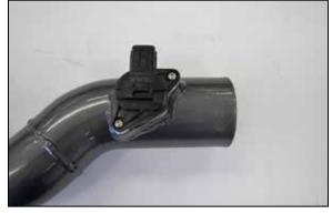
10. Remove the mass air sensor from the factory air filter housing and the install it into the AEM<sup>®</sup> intake tube and secure with the provided hardware.
