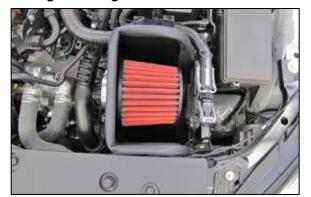
8. Set the AEM<sup>®</sup> air filter into the heat shield assembly.
