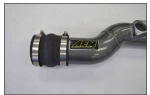
9. Install the provided hump coupler (08487) onto the intake tube and secure with the provided hose clamp.
