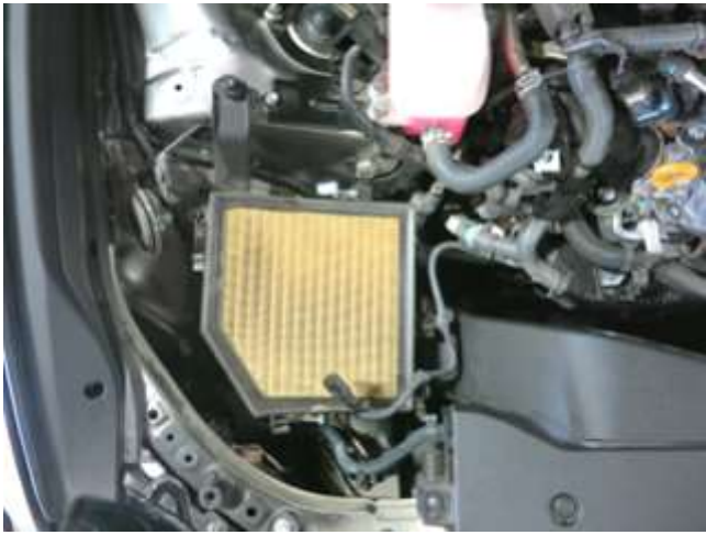
f. Undo the [4] airbox latches and remove the upper intake assembly.
