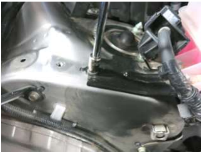
j. Remove the M6 bolt securing the ground cable bracket.
