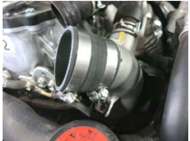
d. Install the coupler with hose clamps onto the turbo inlet pipe. Make sure the smaller end of the coupler is ed to the turbo inlet side. Tighten the hose clamp on the turbo inlet side at this e.
