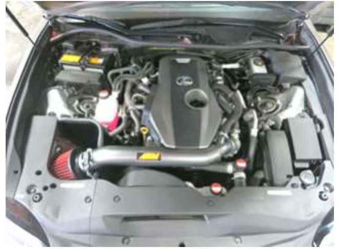
AEM INTAKE INSTALLED
