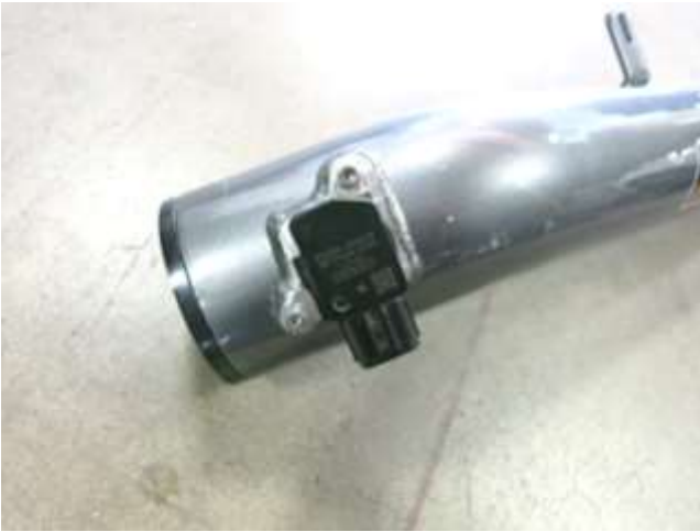
c. Install the MAF sensor using the supplied M4 bolts.
