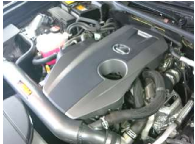
n. Reinstall the engine cover. Make sure the grommets are fully seated.
