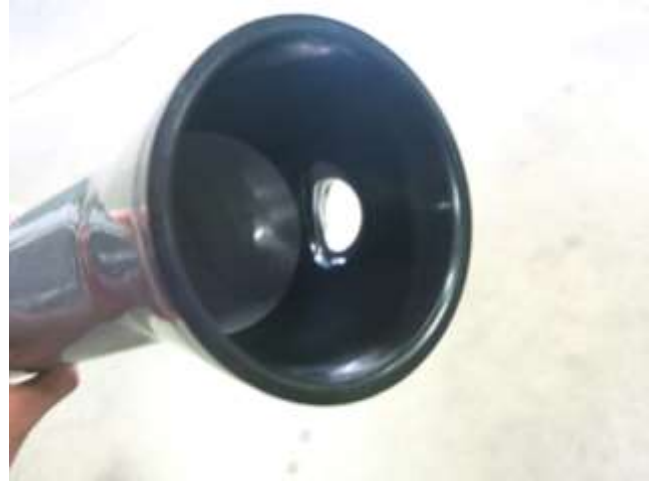
b. Insert the venturi into the intake tube. Be sure to align the pass-thru cutout in the venturi with the hole for the MAF sensor on the AEM intake tube.
