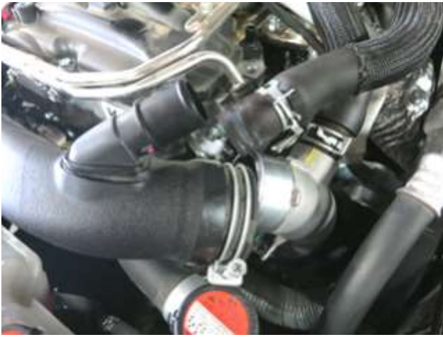
e. Loosen the intake tube hose clamp and pull the PCV hose from the intake tube.
