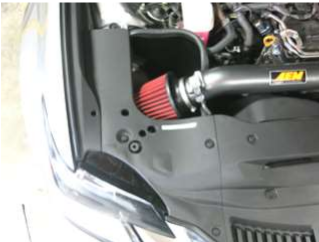
m. Reinstall the plastic shroud with the [4] retainer clips. To reinstall the retainer clips: Pull the mandrel from the main clip, insert the clip into its respective location, and reinsert the mandrel.
