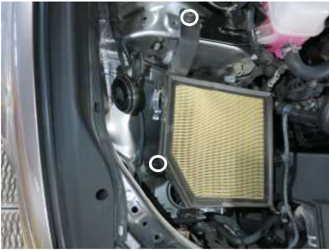
g. Remove the [2] M6 bolts securing the lower airbox.
