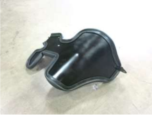
a. Apply the supplied bulb seal trim to the heat shield as shown. Trim as necessary.
