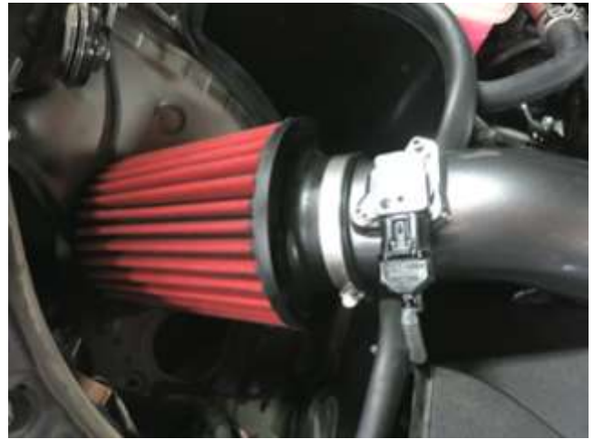
l. Install the AEM air filter and tighten the hose clamp on the air intake tube.
