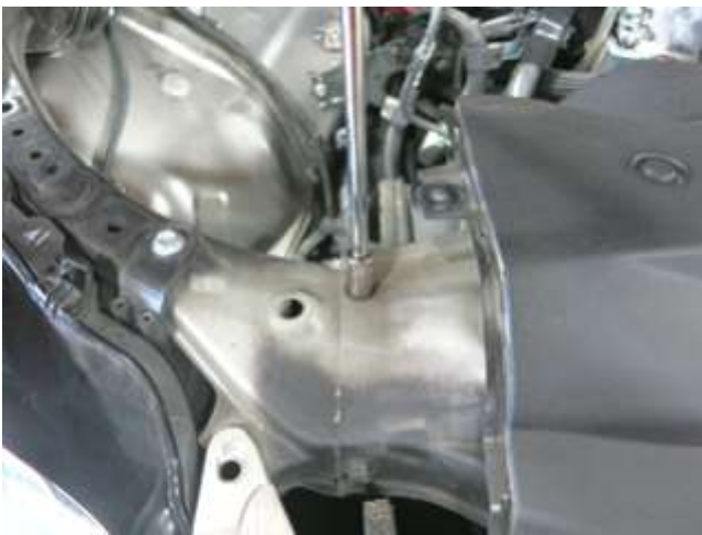
i. Remove the M6 bolt on the core support.
