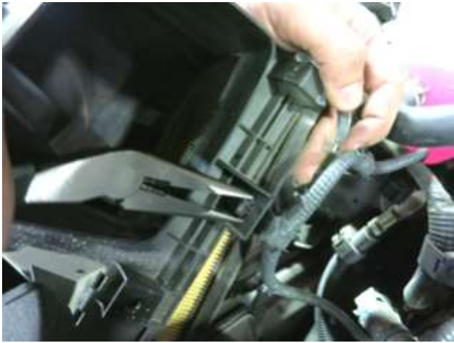
h. Flip the lower airbox around and unclip the MAF harness.
