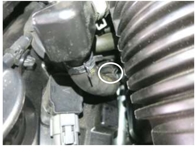
f. Use pliers to release the spring clamp shown above (driver side pictured).
