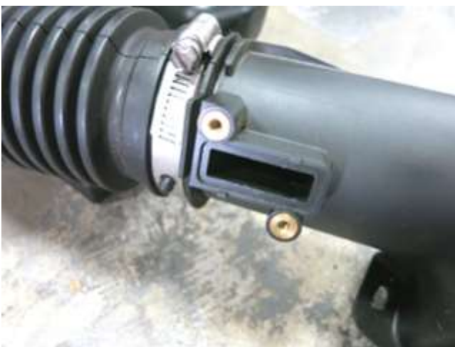
i. Remove the MAF sensor from the intake tube. Repeat for other intake tube.
