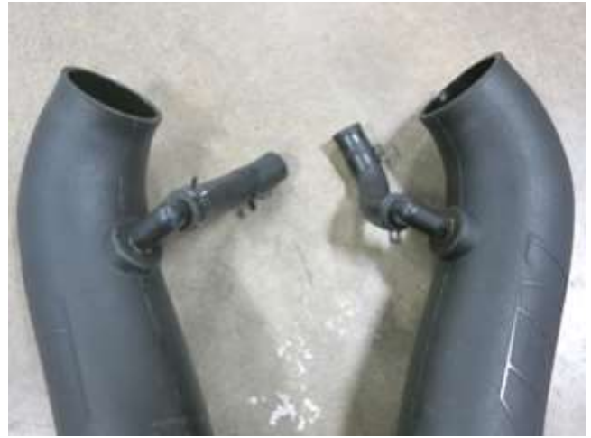
b. Install the plastic 90° fittings into the intake tubes as shown. Do not overtighten. Thread sealant is not required. Install the supplied 5/8" x 5" hose with the [2] factory spring clamps onto one tube. Install the factory breather hose (removed in step 2j) onto the other tube. Orient the hoses as shown.
