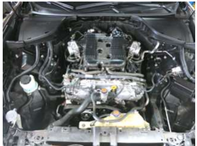
h. Loosen both throttle body hose clamps and the pull both intake tubes and air boxes from the engine bay. Make sure the [4] grommets are still seated in the frame rails.
