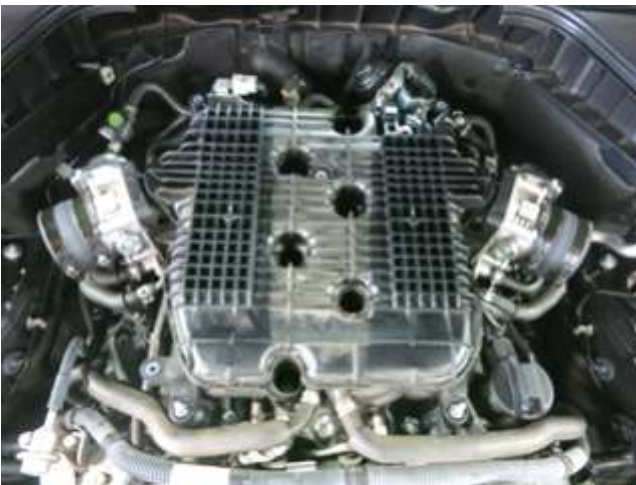
c. Install the [2] couplers along with [4] hose clamps onto the throttle bodies as shown. Tighten the hose clamps on the throttle body side at this time.
