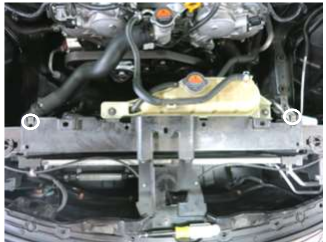
d. Install the [2] clip nuts onto the upper core support in the locations shown above.
