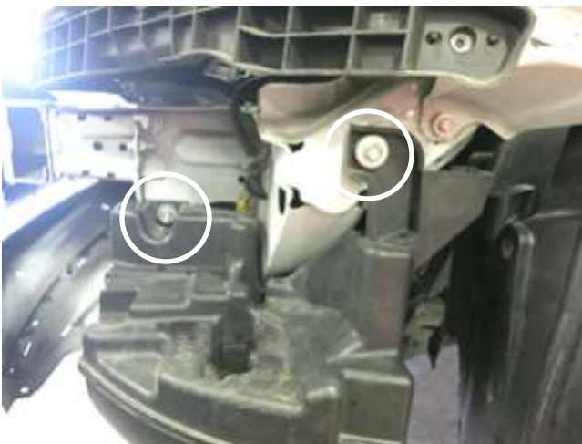
i. Remove the 2 bolts that hold the resonator and remove it from vehicle.
