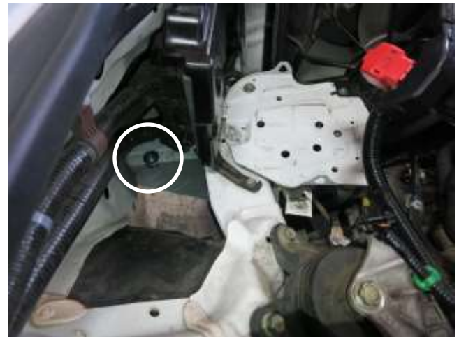
d. Install the supplied 6mm bolt, 2 washers, and 6mm nut into the through hole on the inner fender location shown. NOTE: INSTALL THE BOLT FROM THE BOTTOM SO THE NUT IS ACCESSIBLE FROM THE ENGINE BAY. PLEASE REFER TO THE ILLUSTRATION ON PAGE 2 FOR FURTHER CLARIFICATION.
