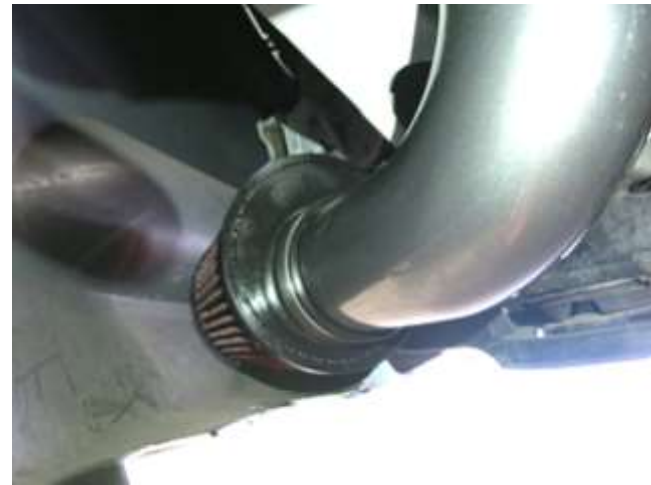
j. Install the AEM Dry W Filter as shown. NOTE: IT MAYBE NECESSARY TO ROTATE THE FILTER UNTIL IT CLEARS ALL NEARBY COMPONENTS.
