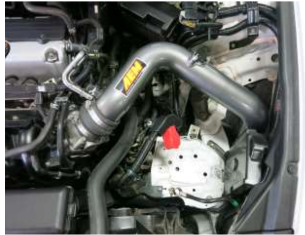
f. Install the intake tube by inserting the bracket to the nut/bolt combo from step 3d, then into the coupler. DO NOT TIGHTEN THE CLAMP AT THIS TIME.
