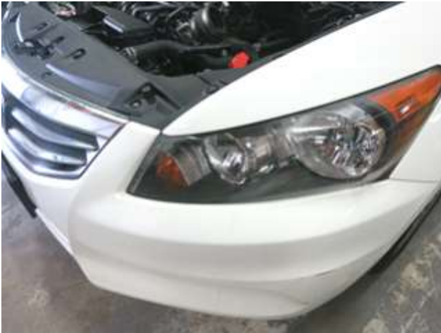
a. Align the front bumper and push into the tabs that support the bumper. Then install all 10mm push clips on the bottom of the bumper.
