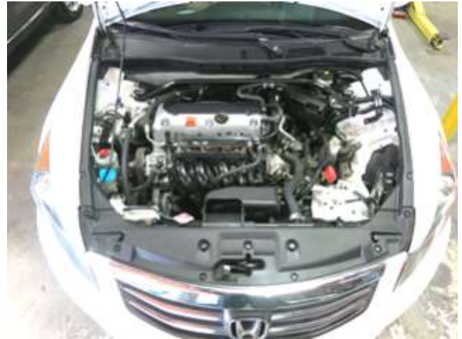
b. Install the core support cover by inserting the 7 10mm clips.
