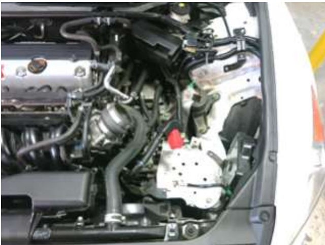
c. Install the coupler onto the throttle body and then only the clamp on the throttle body at this location.
