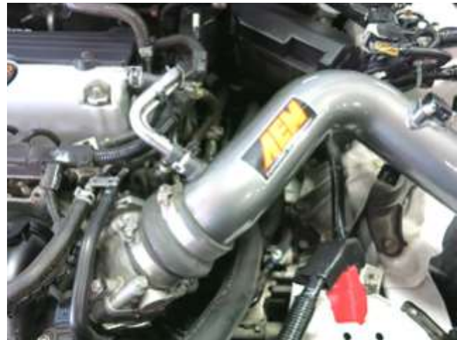
h. Install the supplied PCV nipple to the intake tube then install the PCV line into it. Secure the PCV line with spring clamp from step 2 d.
