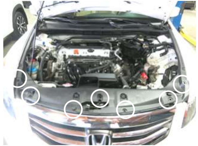
f. Remove the core support cover by releasing the 7 10mm clips.
