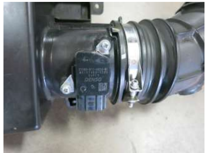
j. Remove the MAF sensor from OE air box. NOTE: MAF SENSOR WILL BE REINSTALLED IN STEP 3e.
