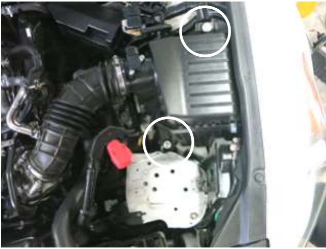
e. Loosen the throttle body clamp and remove the 2 6mm bolts that secure the air box, then remove the complete air box assembly from vehicle.
