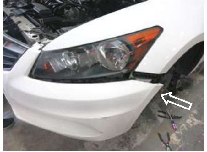
h. Remove all 10mm push clips to remove the bumper to access the resonator by gently pulling the bumper by the wheel well as shown.
