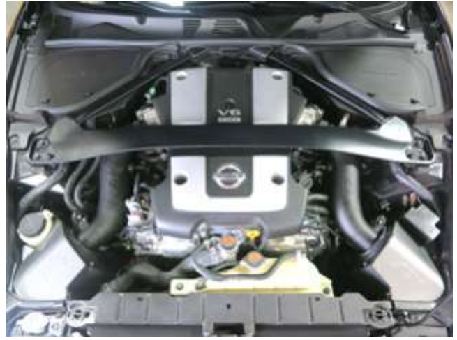
AEM INTAKE INSTALLED
